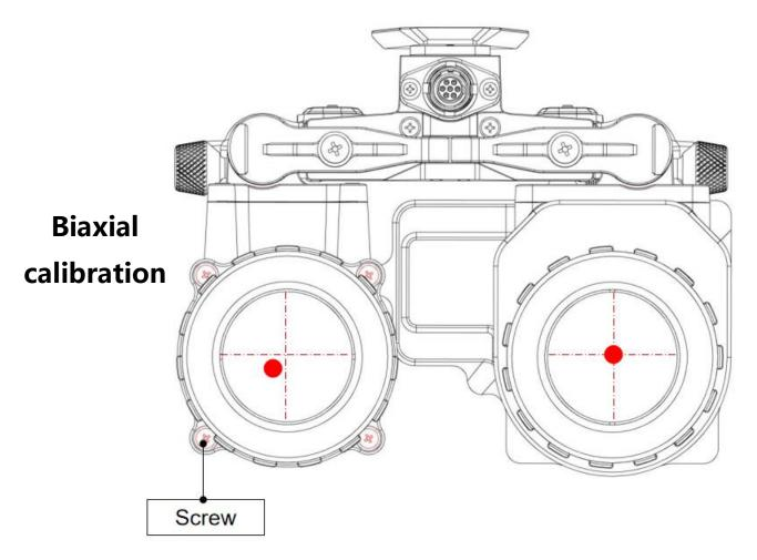
If the whole machine has difficulty in combining images after completing the adjustment of aberration and parallax, and it still cannot be solved after adjusting the visibility of the left and right eyepieces, please loosen the screws of the left eyepiece, and then translate the left eyepiece to achieve the optical axis calibration.
