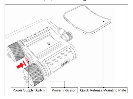
Turn on or off the power of the battery box as shown in the figure (long press). When the battery compartment is powered on, it displays the power (green, blue and red prompts). When it is used, click to display the current power
