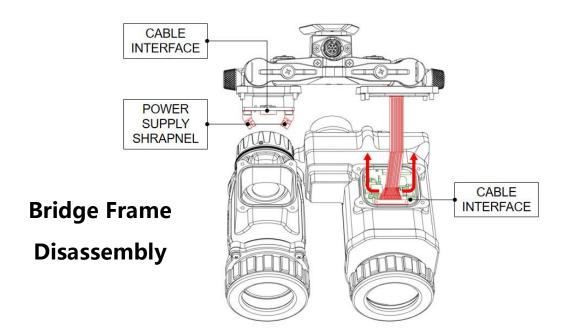
Please remove the PCB cable connector as shown in the figure (please carefully buckle the connector from both ends and do not pull the cable to avoid irreversible device damage)
