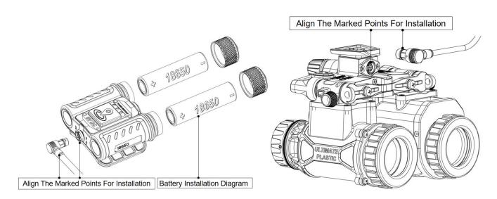
Please complete the installation of battery and cable as shown in the figure. Please use 3.7V standard 18650 battery. Incorrect installation will cause electrical short circuit and equipment damage.
