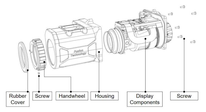
After completing the parallax and aberration adjustment, assemble and restore the components as shown in the figure. (replace the waterproof rubber pad if necessary to achieve sealing effect)
