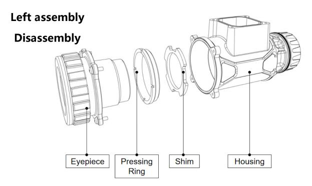
Please disassemble the left eye module as shown in the figure, and remove the eyepiece, pressing ring and shim in turn.
