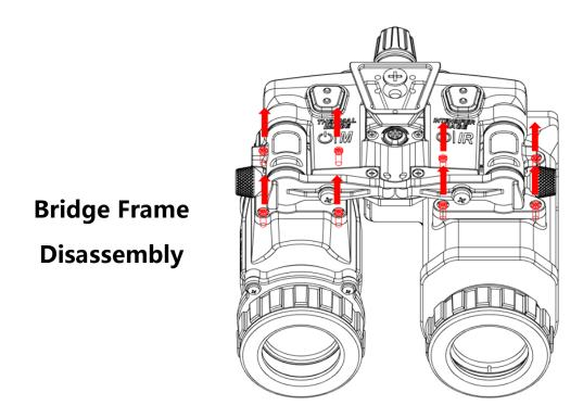
Please remove the left and right assembly screws (PM2-8 pcs.) as shown in the figure
