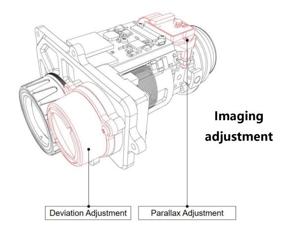
As shown in the figure, the two components are important components for imaging commissioning, Please select a target 35 meters away to complete the adjustment.
