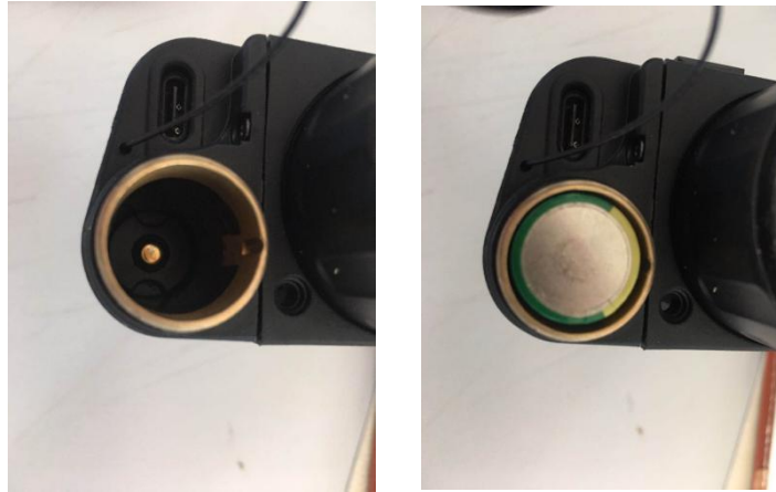
Fig. 5-1 Schematic diagram of battery installation
