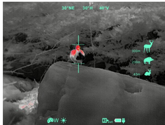
Fig. 6-7 Stadiametric rangefinder interface
