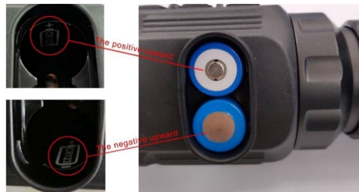
Fig. 8-1 Schematic diagram of battery installation
