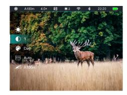
Rotate the **Controller (7)** to select the image contrast option, and press the **Controller (7)** to adjust the image contrast from level 1 to level 5.
