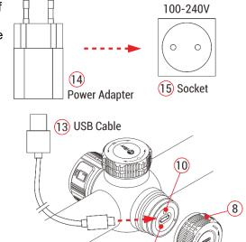
and the LED indicator **(10)** on the device is red. When the indicator **(10)** turns green, it indicates that charging is complete.
