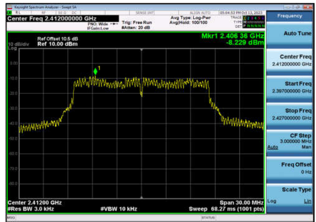
Power spectral density-802.11g ,2462MHz,Ant0
