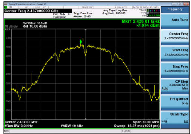
Power spectral density-802.11g ,2412MHz,Ant0
