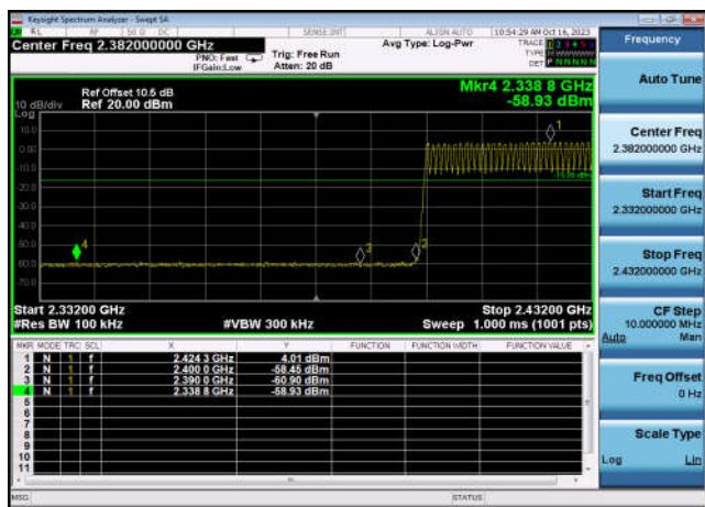
Conducted Emission: DQPSK,2402,2DH5 ,Band Edge
