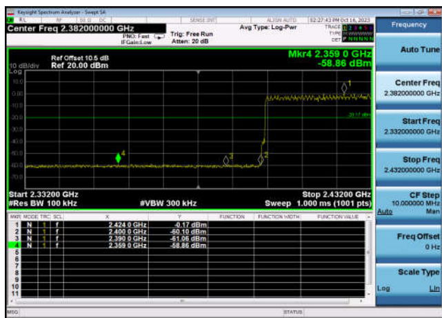
Conducted Emission: 8DPSK,2402,3DH5 ,Band Edge
