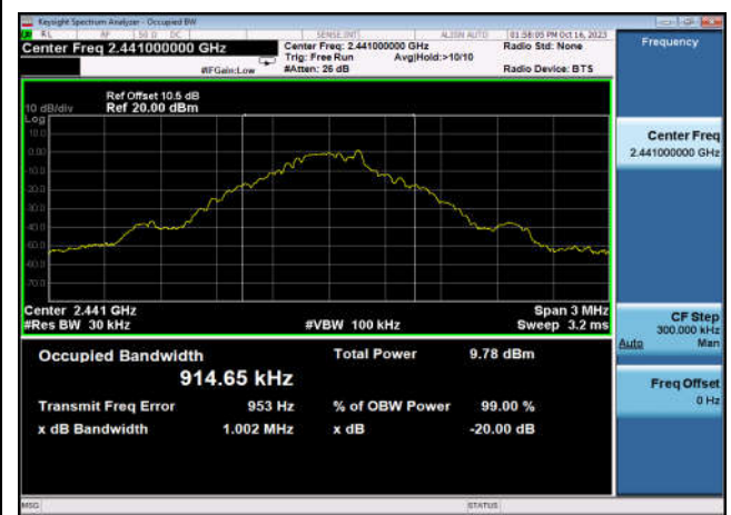
20dB Bandwidth: DQPSK,2402MHz,2DH5
