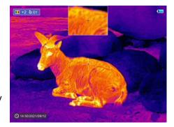
➤ When the main image is enlarged through the shortcut menu, the PIP image will be enlarged 2× synchronously.
