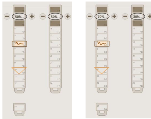
Figure 7.3: Current steering: 50:50 (%) on the left and 70:30 (%) on the right.
