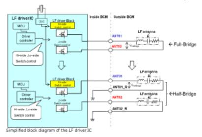
Improper antenna positioning will detune the antenna; drive current may be higher or lower than the current setting or antenna resonant frequency may shift. Please follow the guidelines below to prevent antenna detuning and communication failure during operation.
