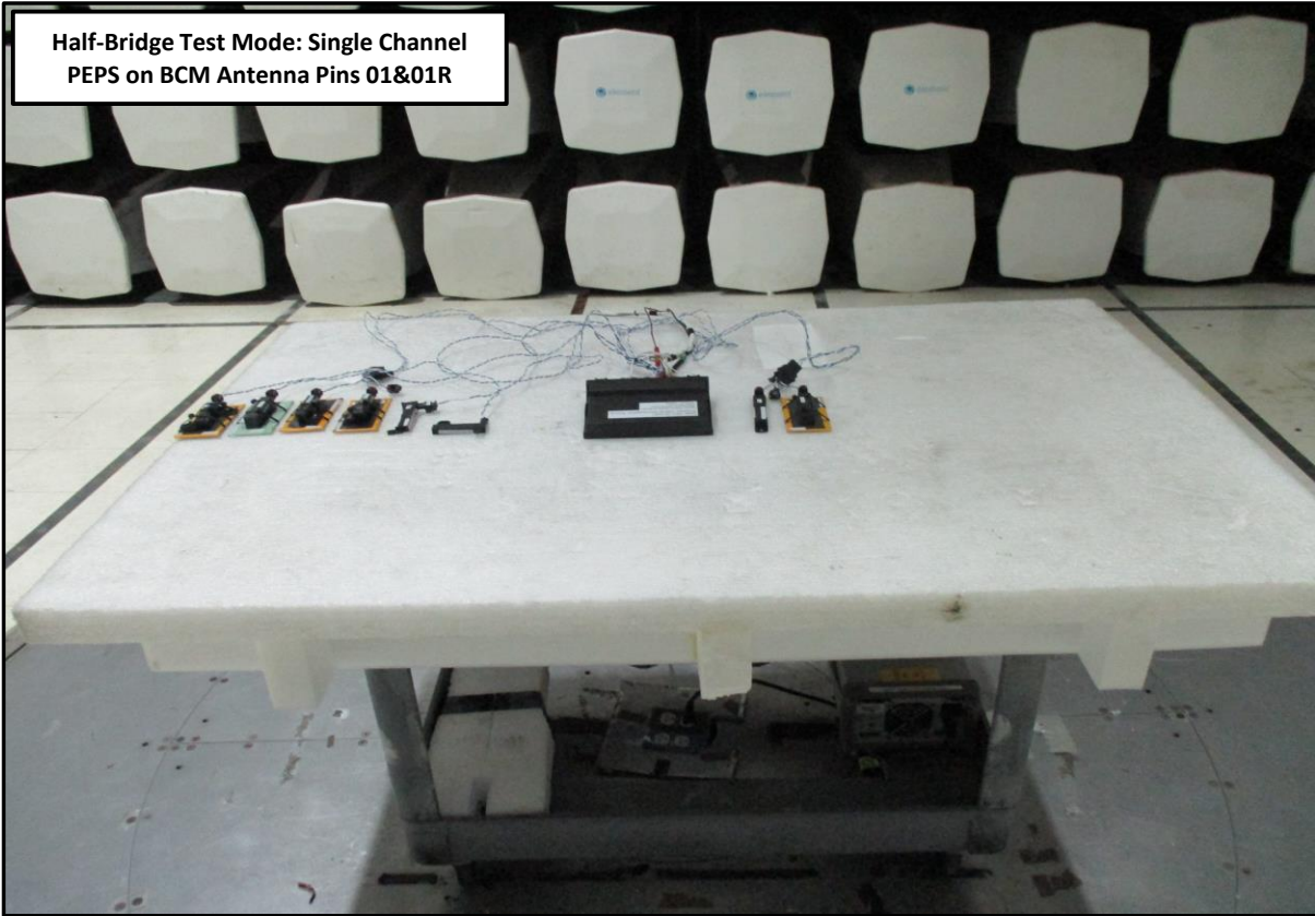
Half-Bridge Test Mode: Single Channel PEPS on BCM Antenna Pins 01&01R
