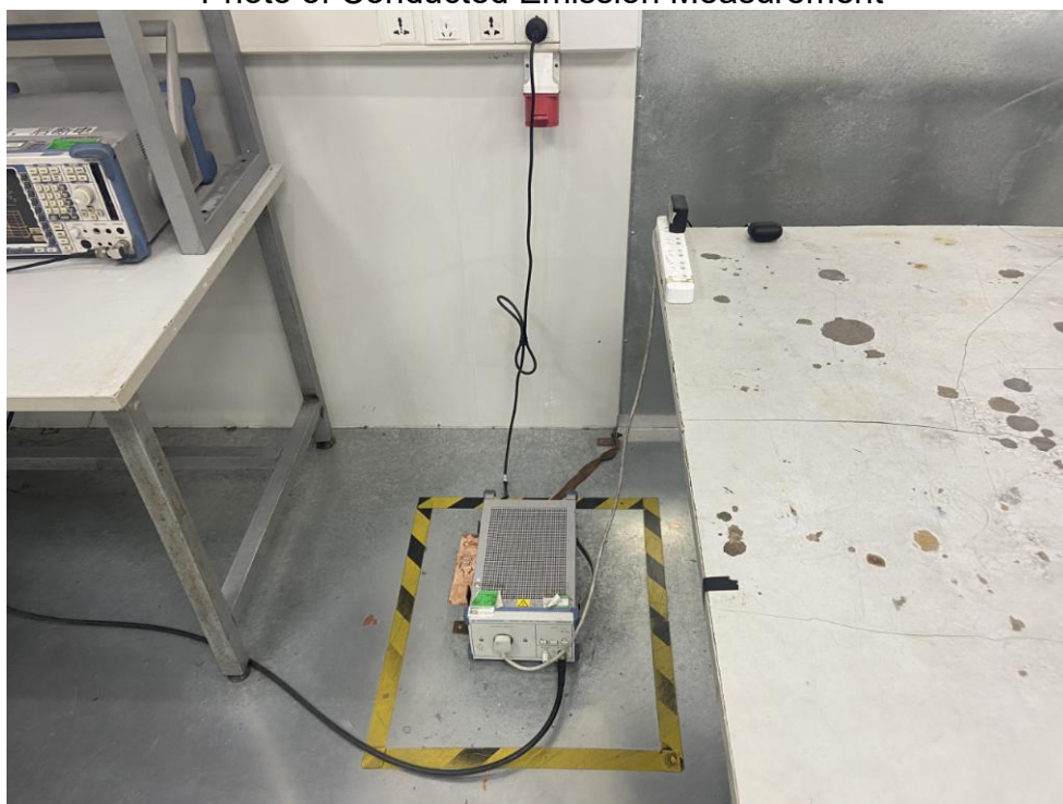
FCC ID: 2AYGN-S5066 Photo of Conducted Emission Measurement
