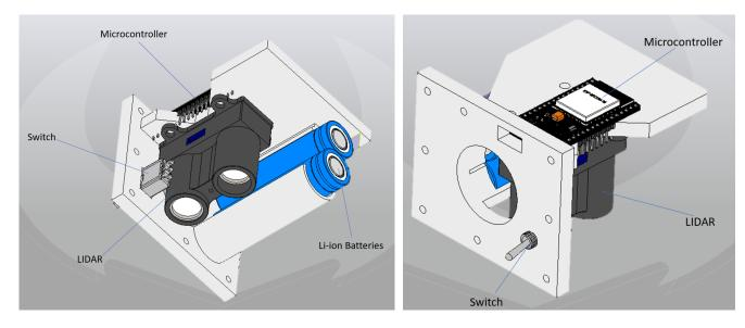
When the switch is flipped up to the "On" position, LEDs on the Microcontroller will light up. The device is programmed so that as soon as it is powered, both the Bluetooth and the IR LIDAR will immediately begin radiating energy in their respective wavelengths.
