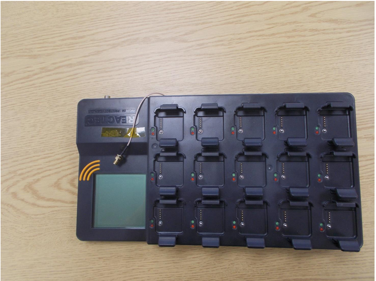
Top view showing temporary antenna connector
