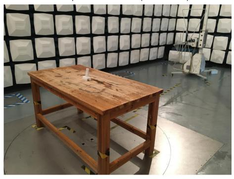
Test Setup For Radiated Emission (Above 1GHz)
