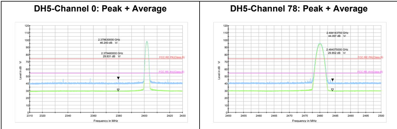
The bandage was performed in all EDR mode(2DH5 and 3DH5), 3DH5 was selected as the worse condition. The test data of the worst-case condition was recorded in this report.
