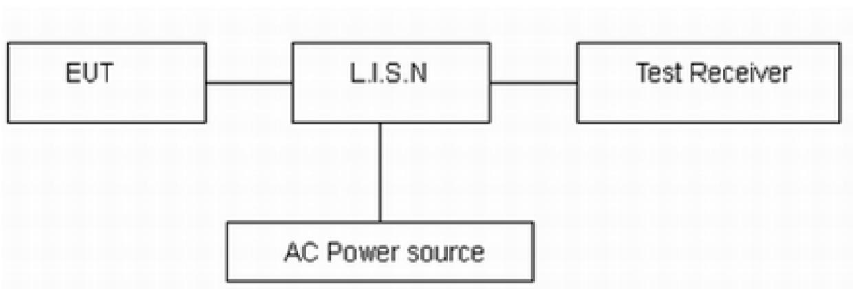
Note: AC Power source is used to 120V/60Hz.
