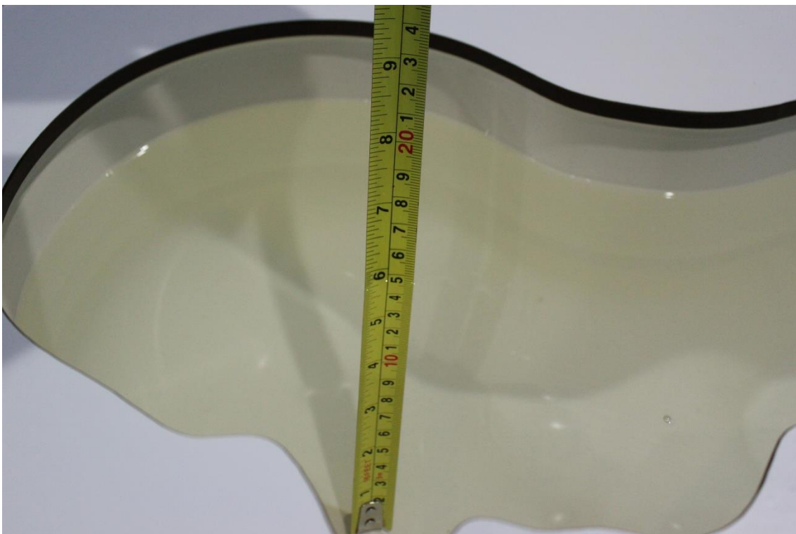
Picture 8-5 Liquid depth in the Head Phantom (5GHz)
