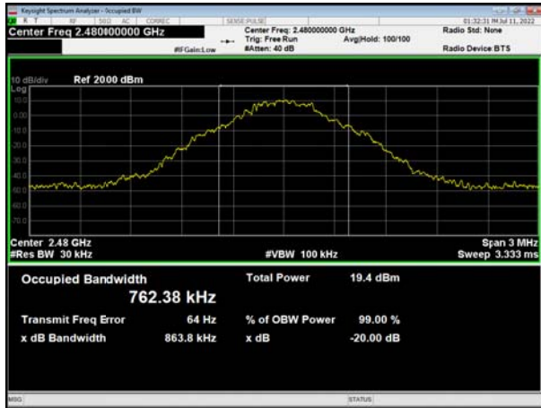
BT DH5 CH78, Carrier frequency (MHz): 2480
