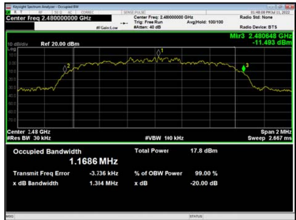
BT 2DH5 CH78, Carrier frequency (MHz): 2480
