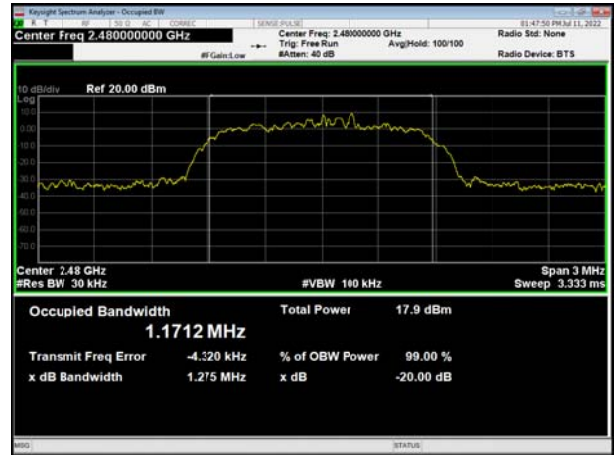
BT 2DH5 CH78, Carrier frequency (MHz): 2480
