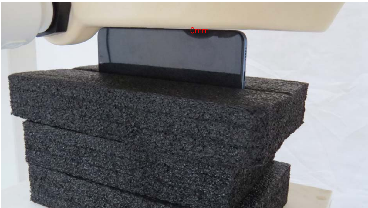
Picture 16: Right Edge, the distance from handset to the bottom of the Phantom is 0mm
