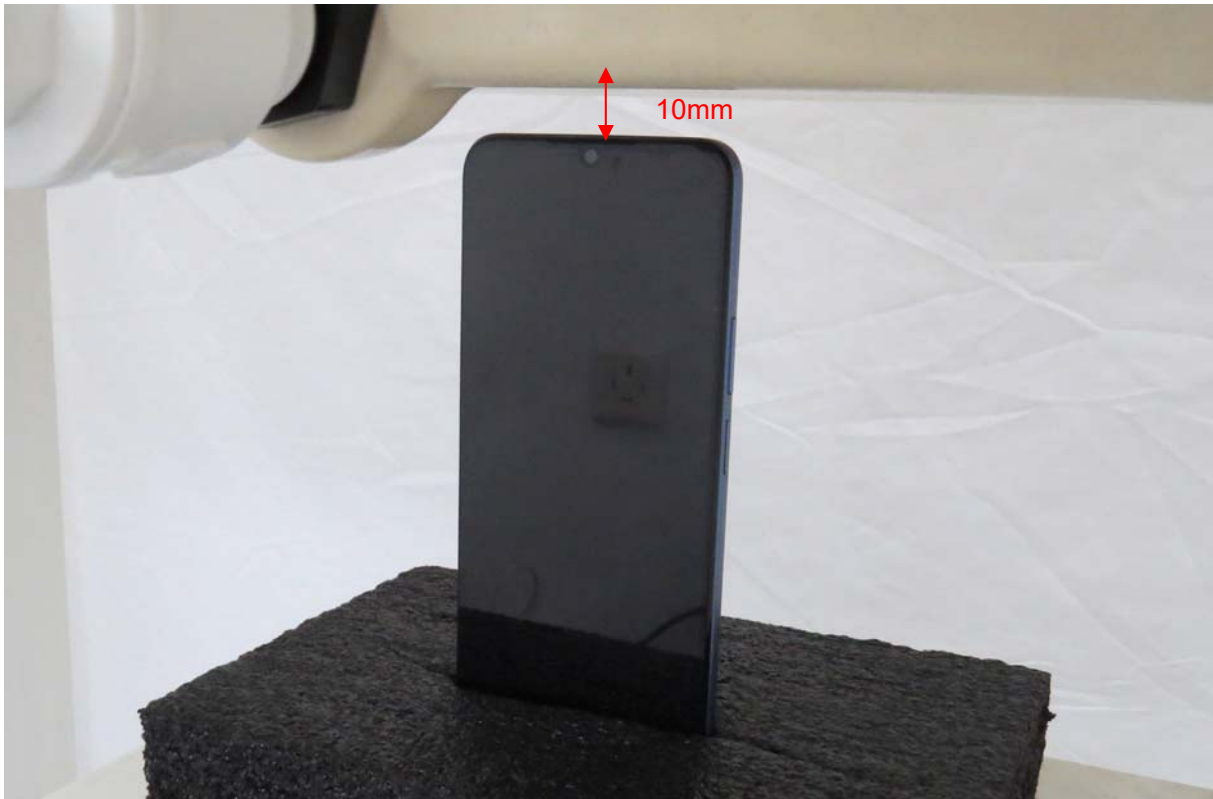
Picture 11: Top Edge, the distance from handset to the bottom of the Phantom is 10mm
