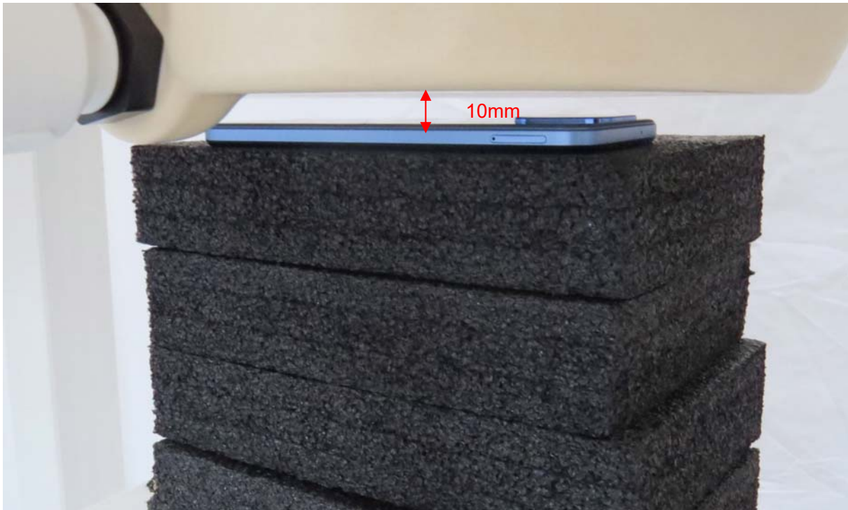
Picture 7: Back Side, the distance from handset to the bottom of the Phantom is 10mm
