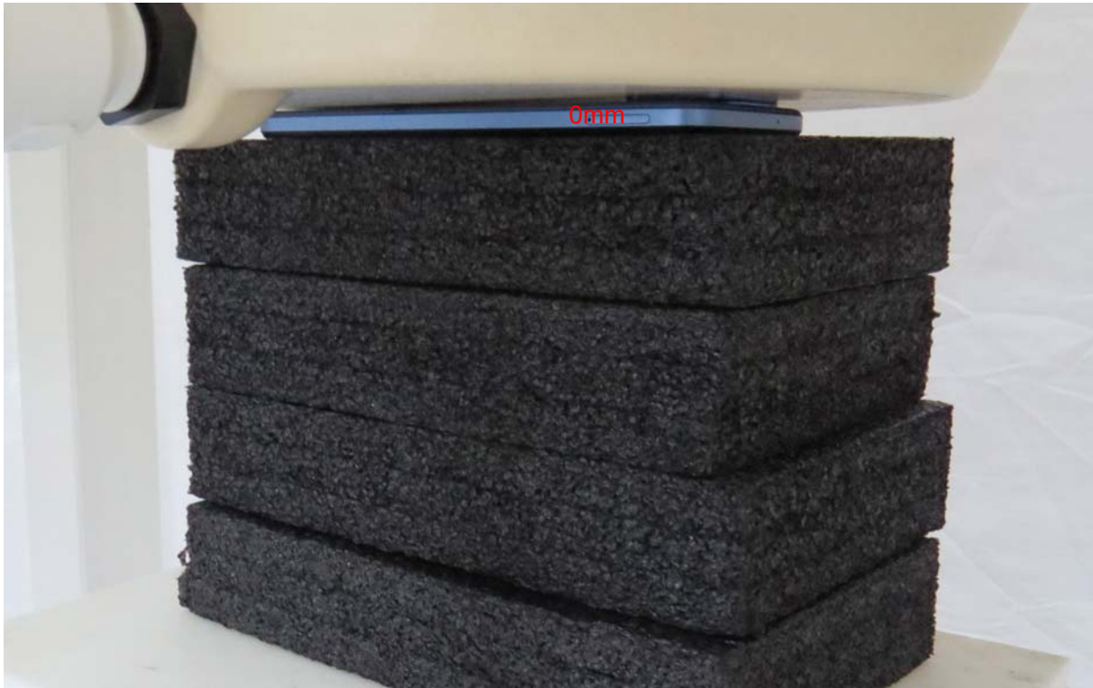
Picture 13: Back Side, the distance from handset to the bottom of the Phantom is 0mm
