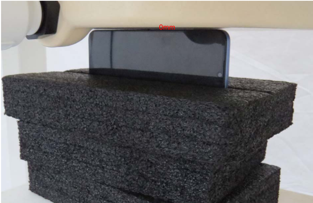
Picture 15: Left Edge, the distance from handset to the bottom of the Phantom is 0mm
