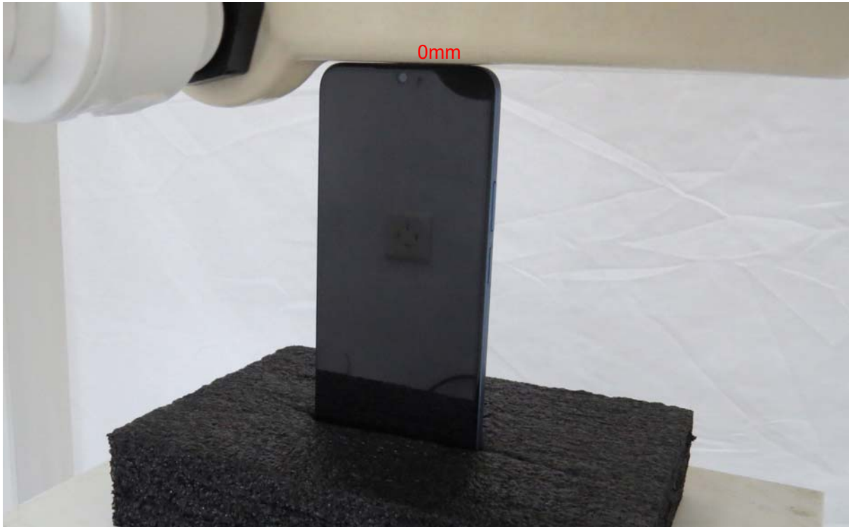
Picture 17: Top Edge, the distance from handset to the bottom of the Phantom is 0mm
