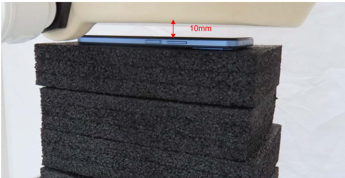
Picture 8: Front Side, the distance from handset to the bottom of the Phantom is 10mm
