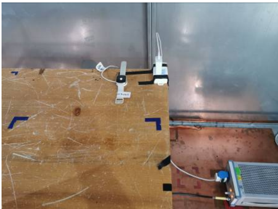
Conducted Emissions Test Setup
