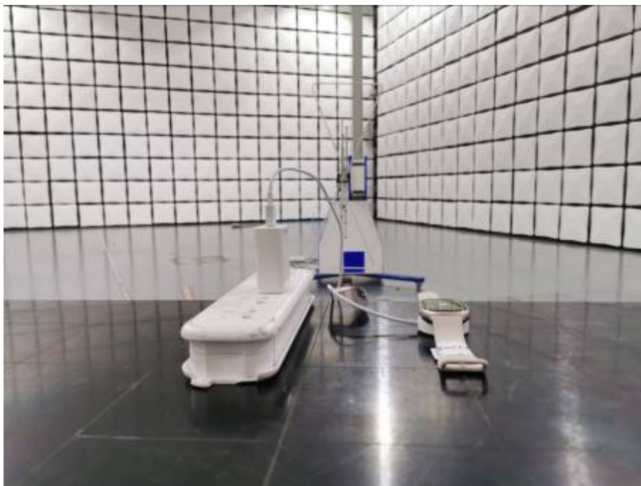
Radiated Emissions Test Setup (30-1000MHz)
