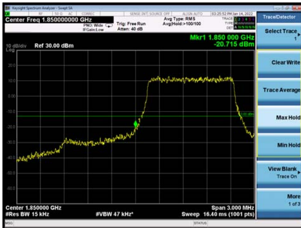
LTE Band 2 3MHz QPSK 1RB CH-Low
