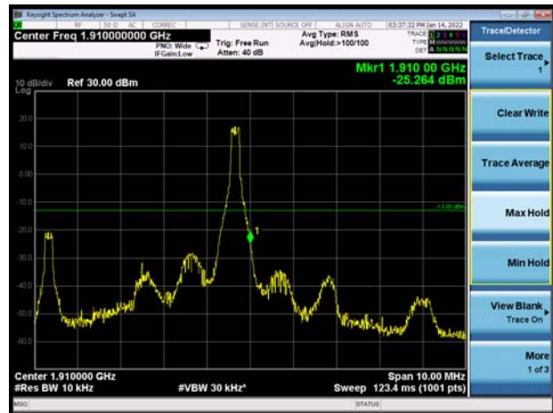
LTE Band 2 5MHz QPSK 100%RB CH-High
