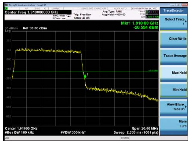
LTE Band 2 15MHz 16QAM 1RB CH-High
