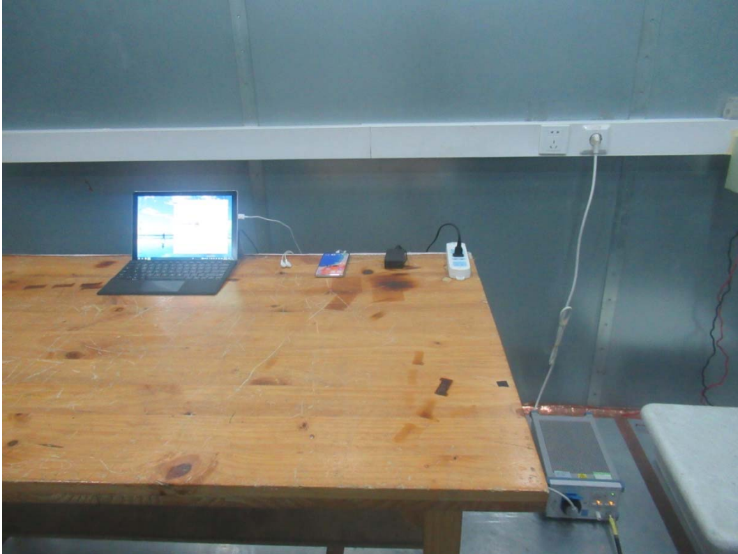
Picture 2: Conducted Emissions Test Setup
