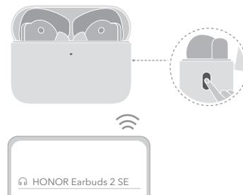
EN Open the charging case. Press and hold the Function button for 2s until the indicator flashes white. The earphones then enter Pairing mode. The earphones will automatically enter Pairing mode when powered on for the first time.
