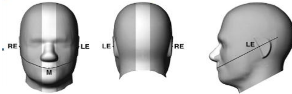
F-3. Front, back, and side views of SAM (model for the phantom shell). Full-head model is for illustration purposes only—procedures in this recommended practice are intended primarily for the phantom setup.
