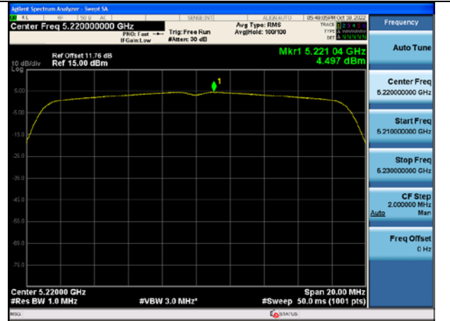
Test Mode:802.11ac VHT20 5220MHz Chain0
