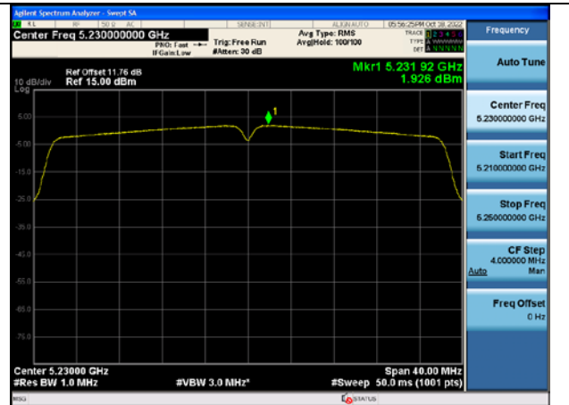
Test Mode:802.11ac VHT40 5230MHz Chain0
