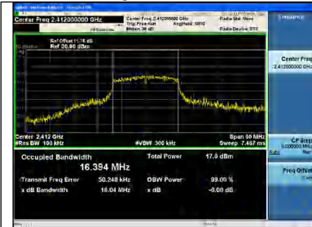
Test Mode:802.11g 2412MHz Chain0
