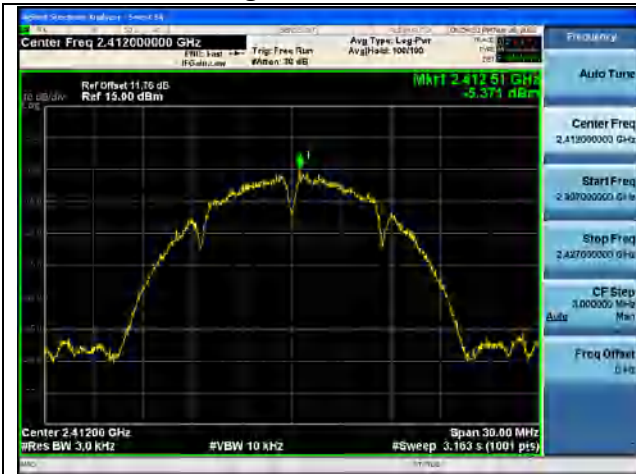
Test Mode:802.11g 2412MHz Chain0
