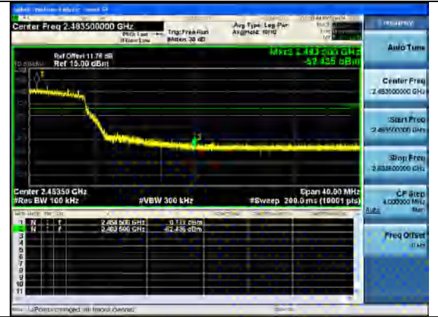
Test Mode:802.11g 2462MHz Chain0
