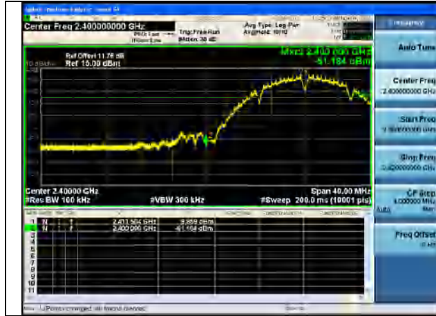
Test Mode:802.11b 2412MHz Chain0
