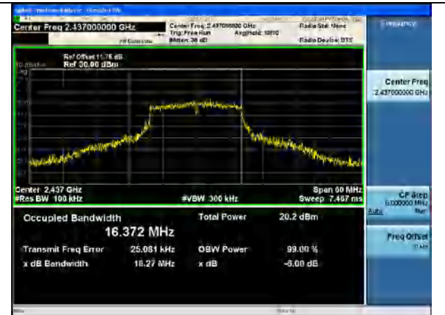
Test Mode:802.11g 2437MHz Chain0
