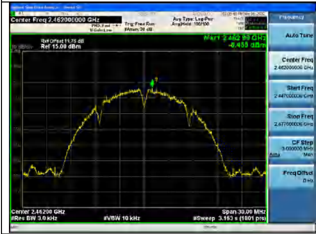
Test Mode:802.11g 2462MHz Chain0
