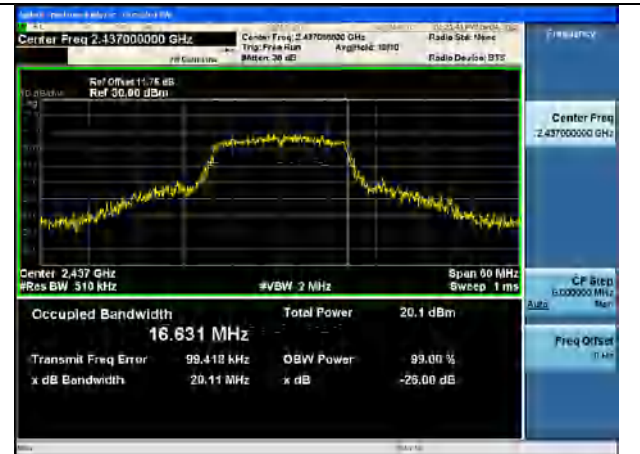
Test Mode:802.11g 2437MHz Chain0
