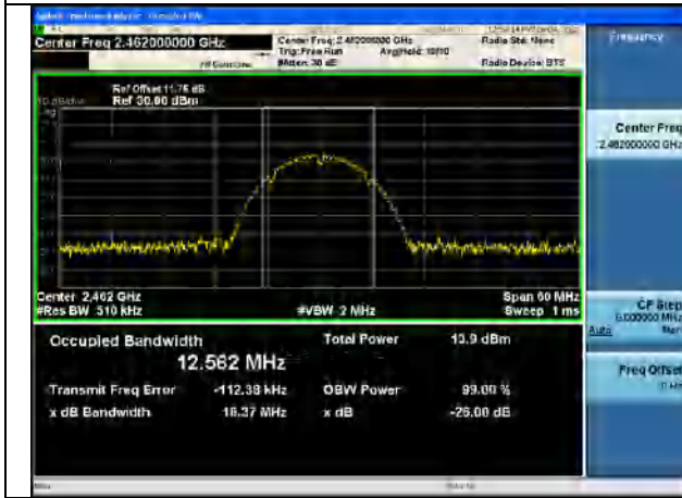
Test Mode:802.11b 2462MHz Chain0
