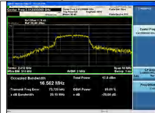
Test Mode:802.11g 2412MHz Chain0
