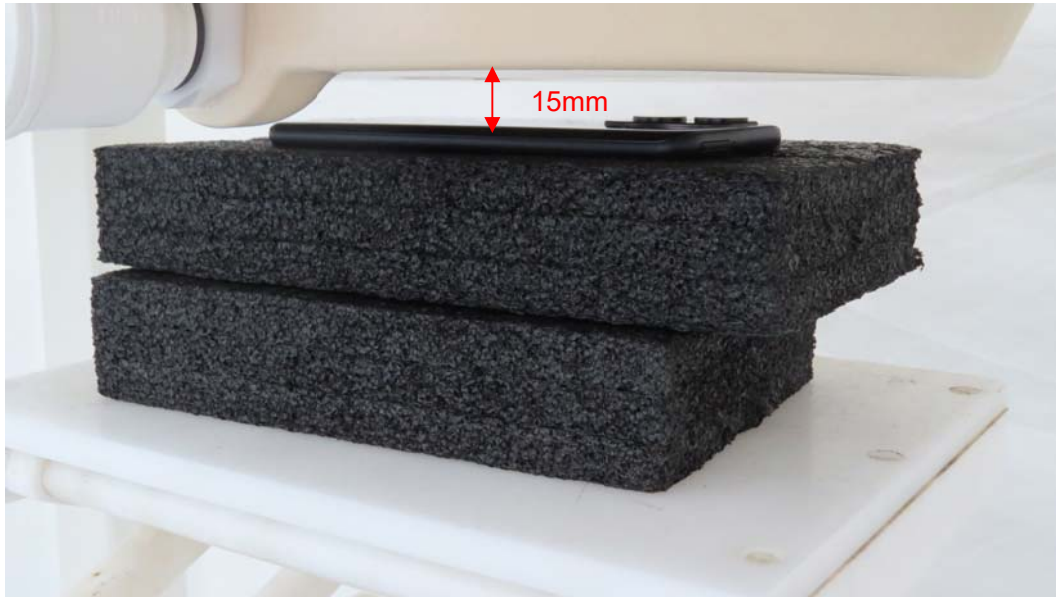
Picture 5: Back Side, the distance from handset to the bottom of the Phantom is 15mm
