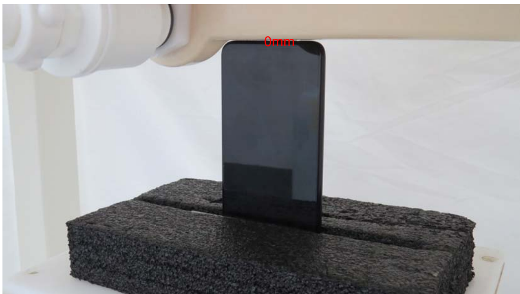
Picture 18: Bottom Edge, the distance from handset to the bottom of the Phantom is 0mm
