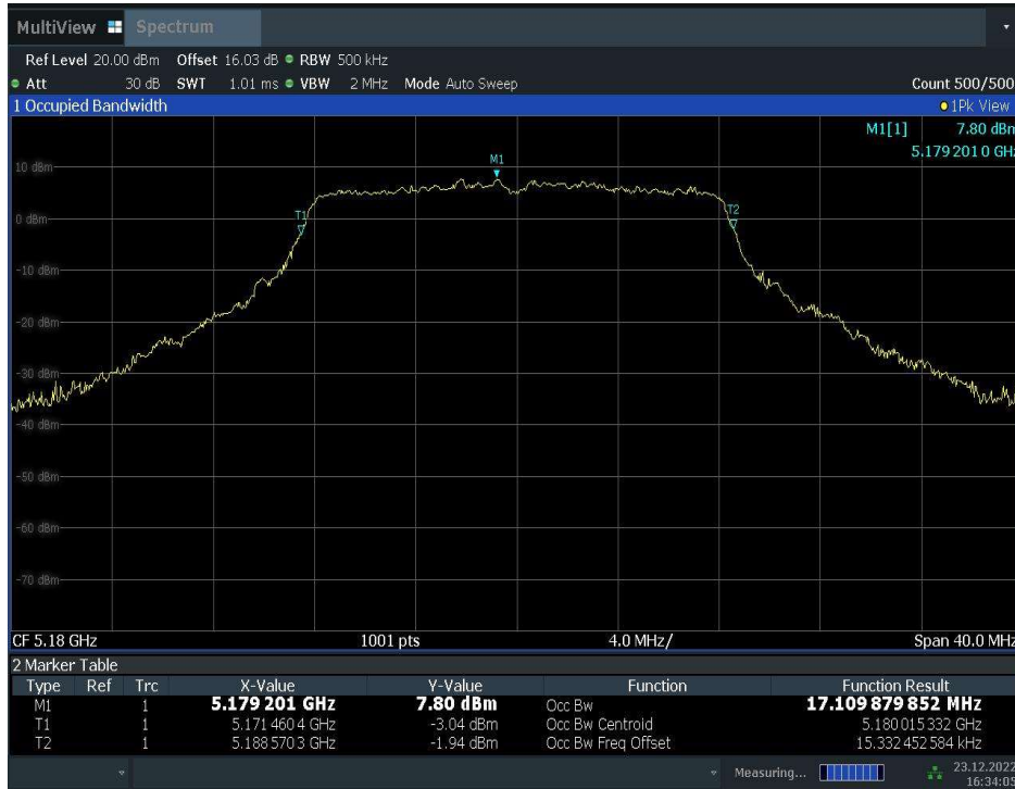
Fig.34 99% Occupied bandwidth (802.11a, 5180MHz)
