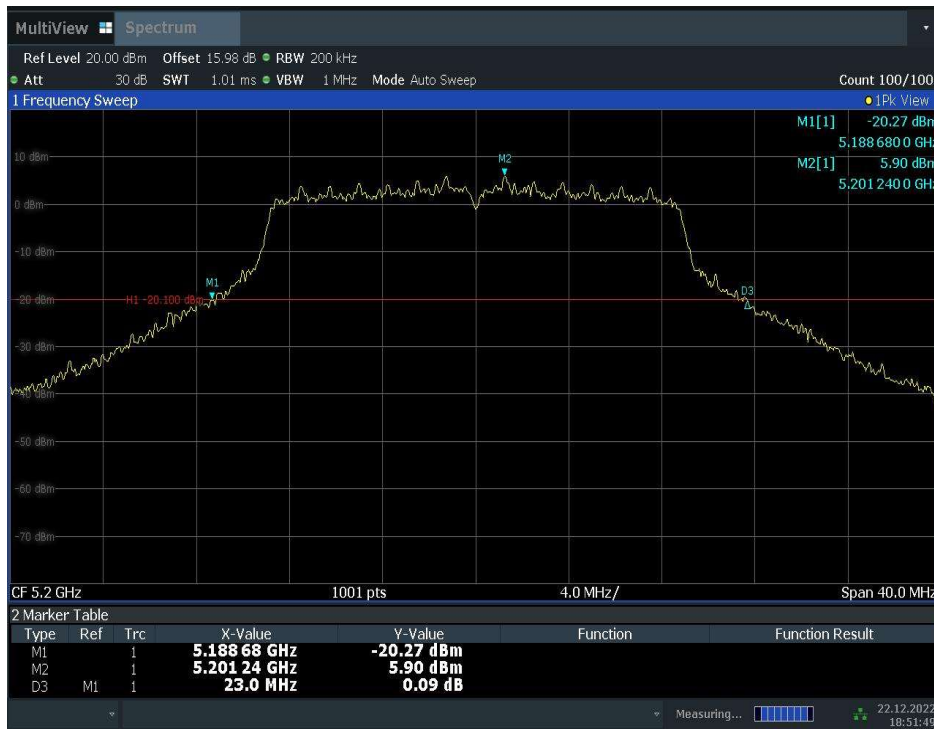
Fig.12 Occupied 26dB Bandwidth (802.11ac-VHT20, 5200MHz)
