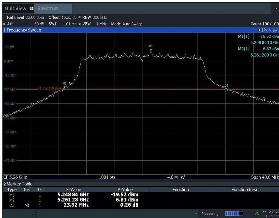
Fig.14 Occupied 26dB Bandwidth (802.11ac-VHT20, 5260MHz)
