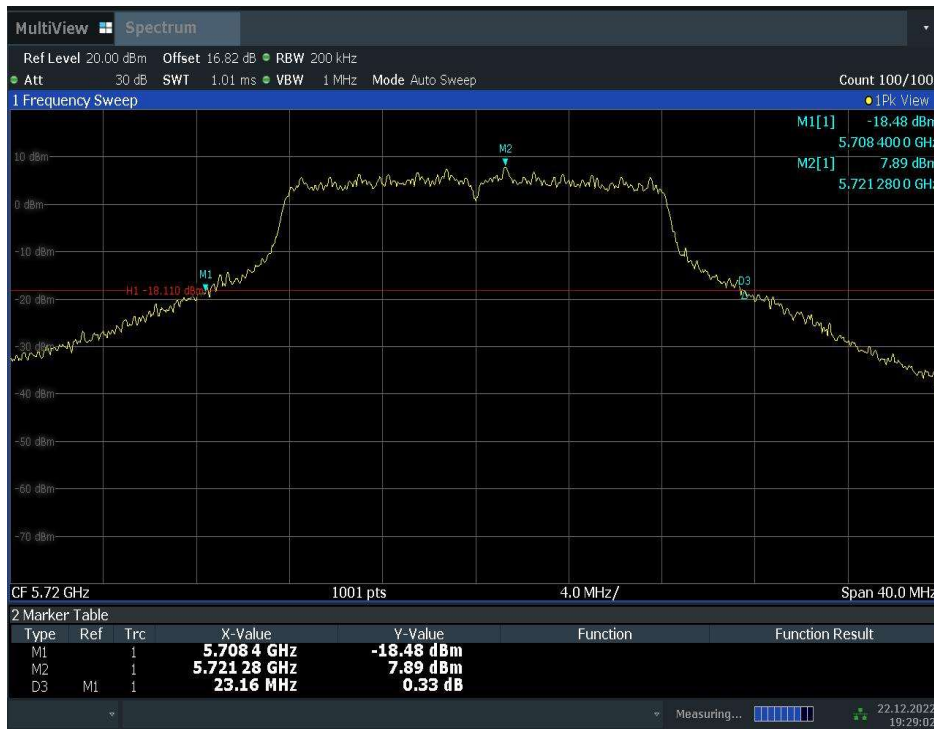
Fig.10 Occupied 26dB Bandwidth (802.11a, 5720MHz)
