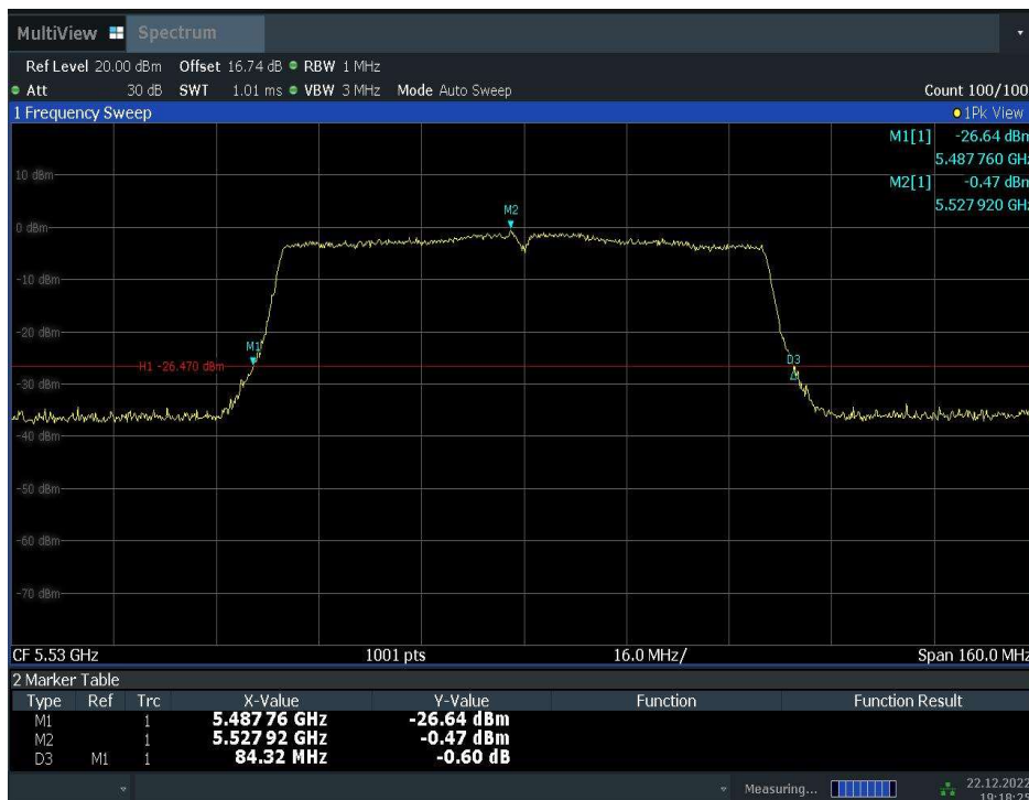
Fig.31 Occupied 26dB Bandwidth (802. 11ac-VHT80, 5530MHz)
