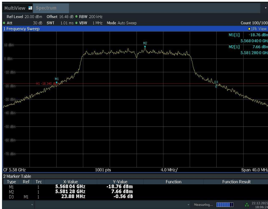
Fig.8 Occupied 26dB Bandwidth (802.11a, 5580MHz)
