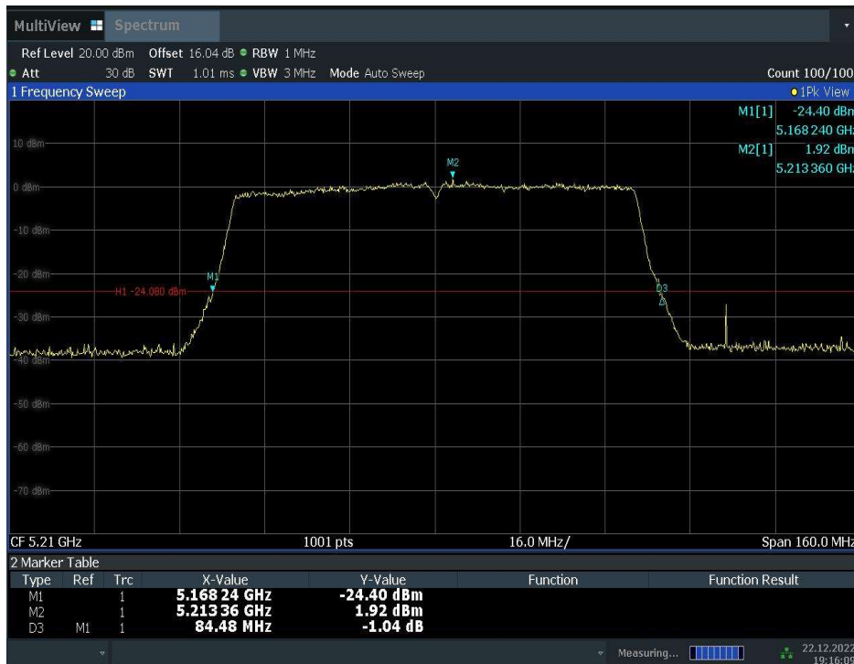
Fig.29 Occupied 26dB Bandwidth (802. 11ac-VHT80, 5210MHz)
