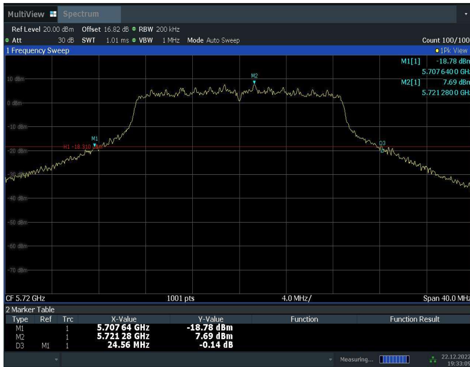
Fig.20 Occupied 26dB Bandwidth (802. 11ac-VHT20, 5720MHz)
