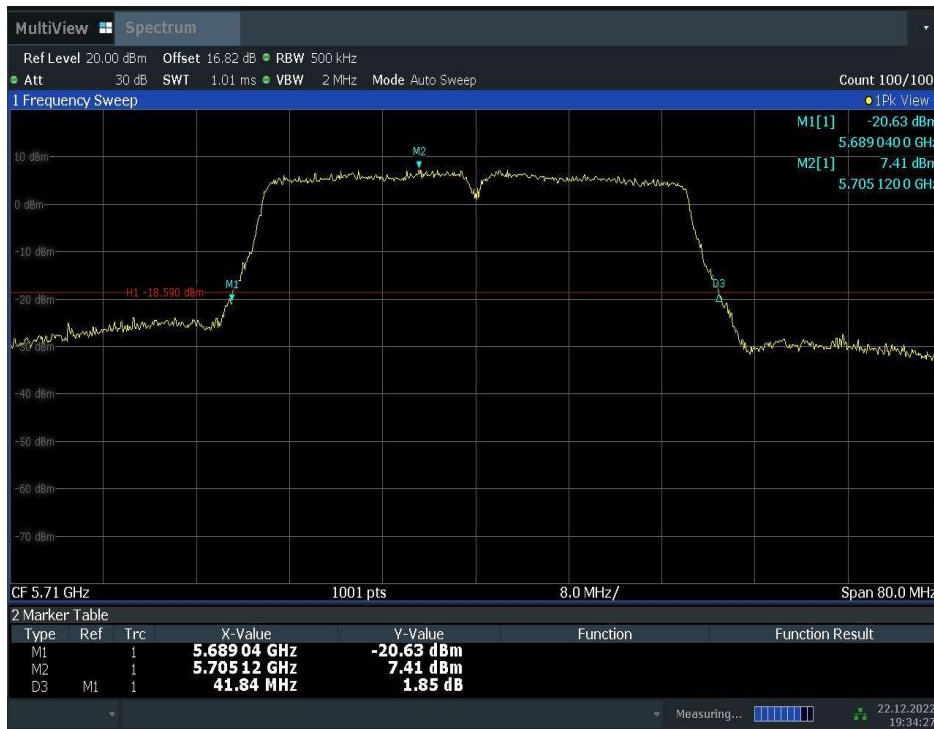
Fig.28 Occupied 26dB Bandwidth (802. 11ac-VHT40, 5710MHz)
