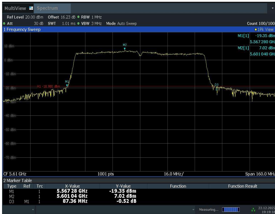
Fig.32 Occupied 26dB Bandwidth (802. 11ac-VHT80, 5610MHz)
