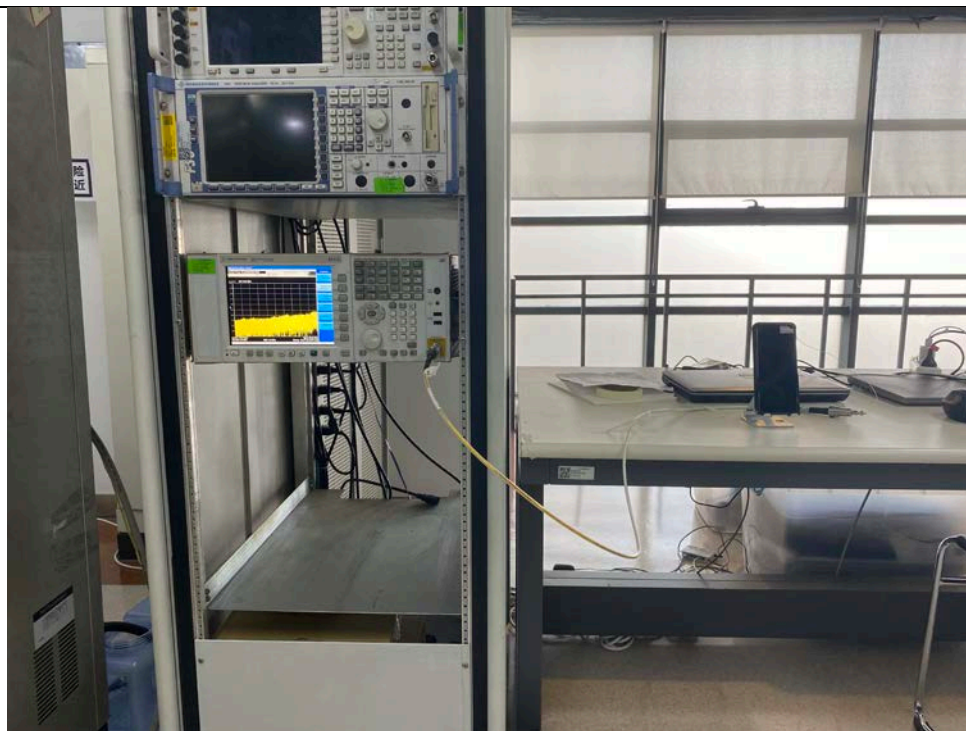
RF Conducted Test setup (BT/WIFI)
