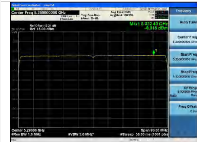
Test Mode:802.11ax HE80 5290MHz Chain0
