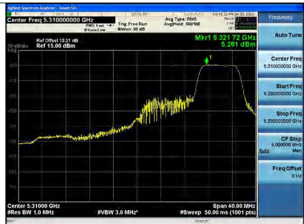
Test Mode:802.11be HE40 5310MHz Chain0
