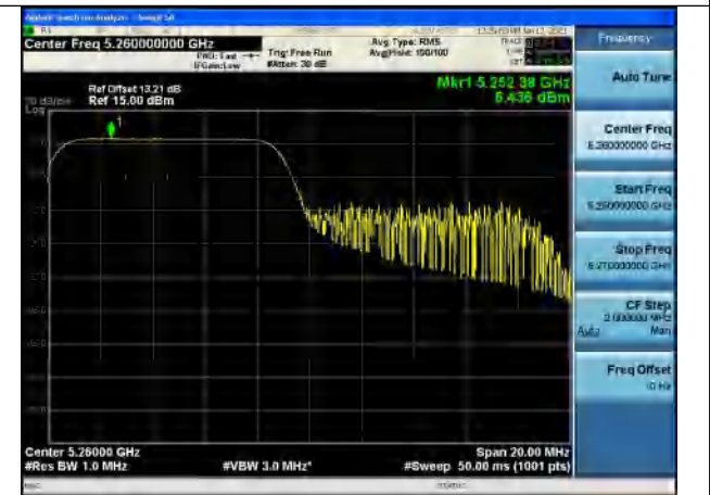
Test Mode:802.11be EHT20 5260MHz Chain1
