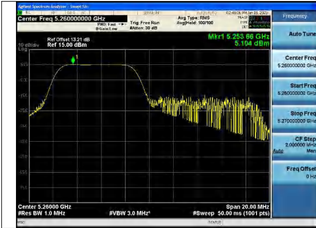
Test Mode:802.11be HE20 5260MHz Chain0
