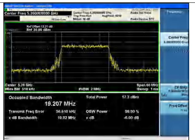
Test Mode:802.11be EHT20 5260MHz Chain1
