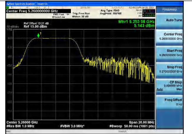
Test Mode:802.11be HE20 5260MHz Chain1
