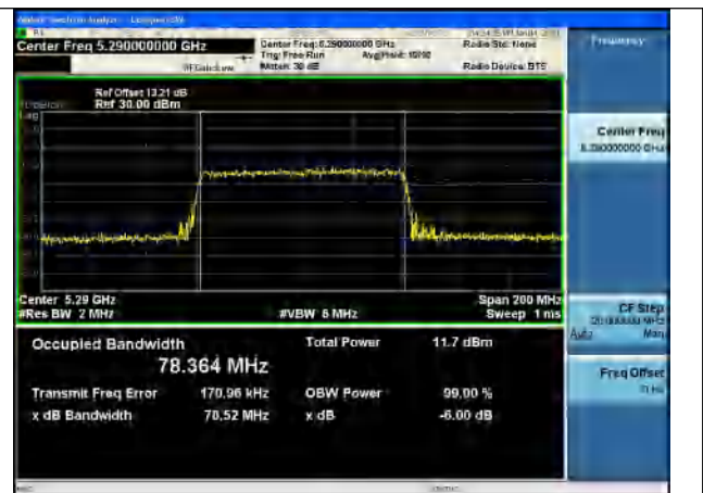
Test Mode:802.11ax HE80 5290MHz Chain1
