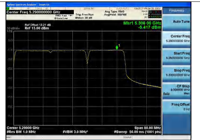
Test Mode:802.11be HE80 5290MHz Chain1
