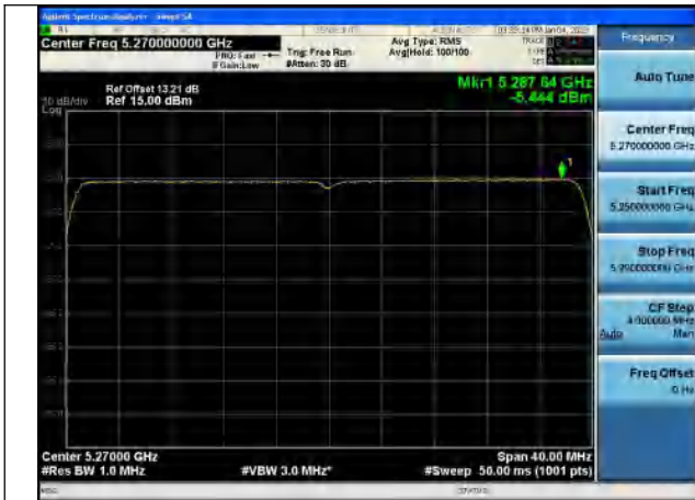
Test Mode:802.11ax HE40 5270MHz Chain1
