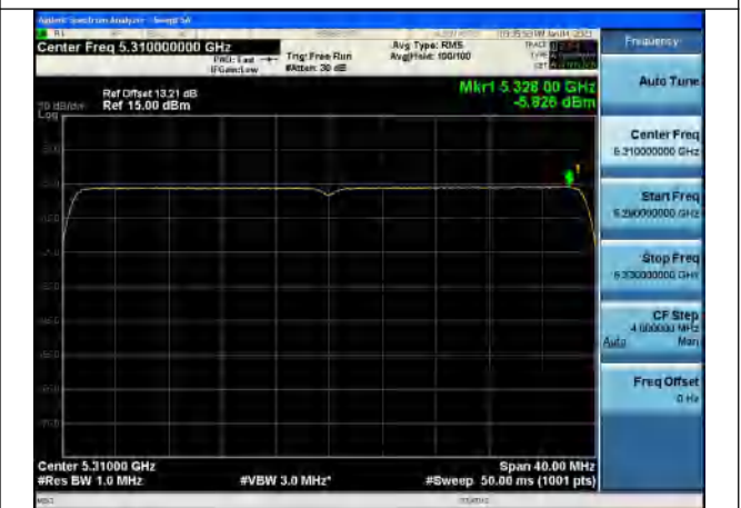
Test Mode:802.11ax HE40 5310MHz Chain0
