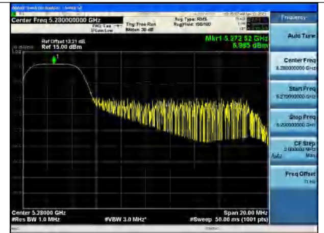
Test Mode:802.11be EHT20 5280MHz Chain0
