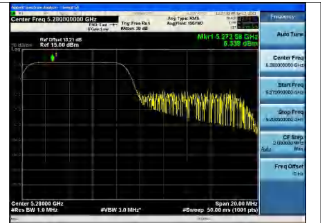
Test Mode:802.11be EHT20 5280MHz Chain0
