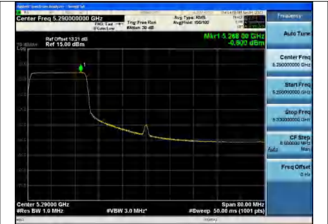
Test Mode:802.11ax HE80 5290MHz Chain1
