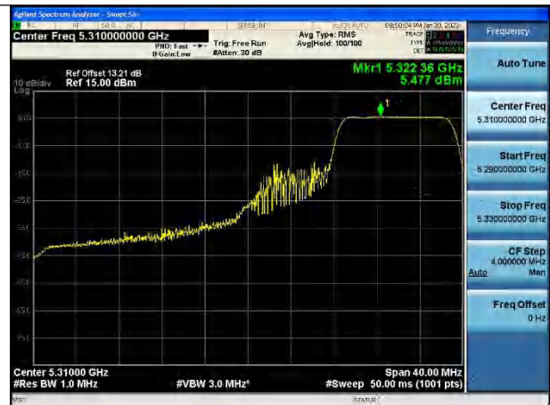
Test Mode:802.11be HE40 5310MHz Chain1
