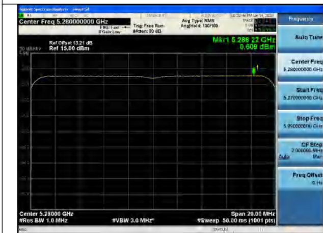
Test Mode:802.11ax HE20 5280MHz Chain1
