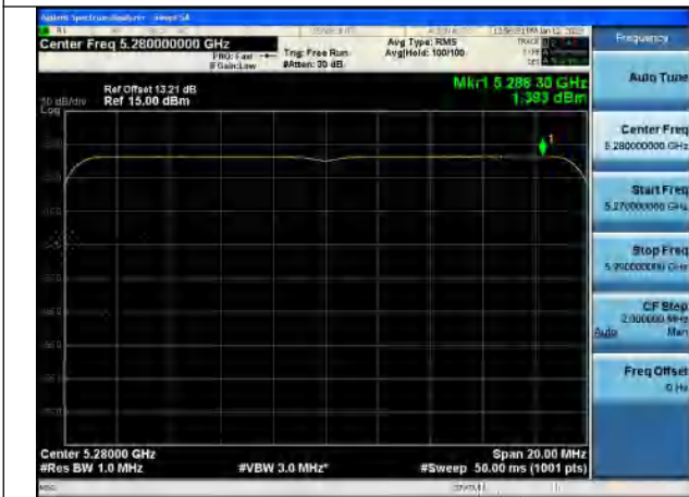
Test Mode:802.11be EHT20 5280MHz Chain1
