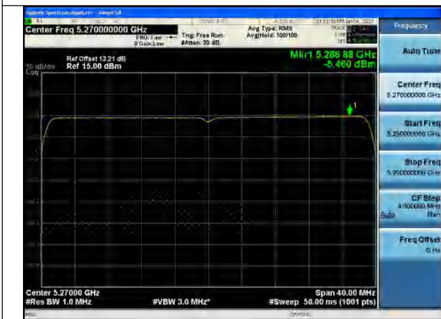
Test Mode:802.11ax HE40 5270MHz Chain0
