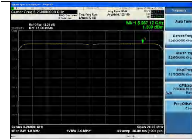
Test Mode:802.11be EHT20 5260MHz Chain0
