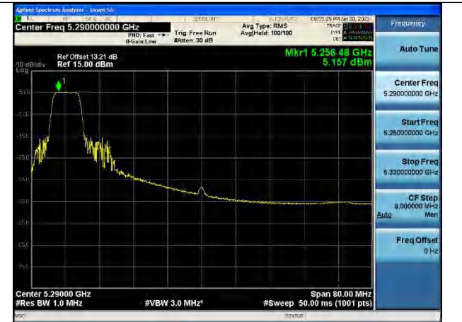
Test Mode:802.11be HE80 5290MHz Chain1
