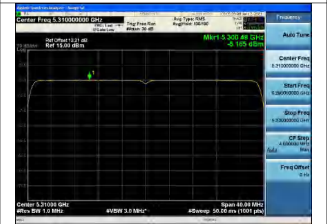
Test Mode:802.11be EHT40 5310MHz Chain0
