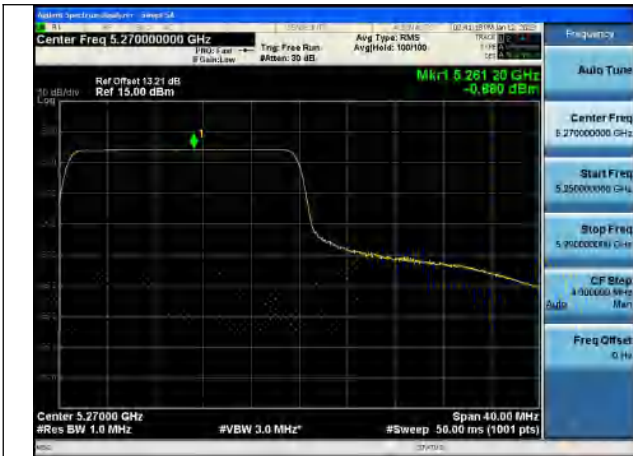
Test Mode:802.11be EHT40 5270MHz Chain0
