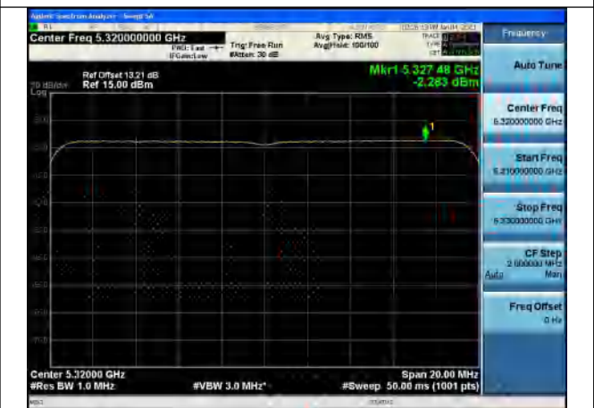
Test Mode:802.11ax HE20 5320MHz Chain1
