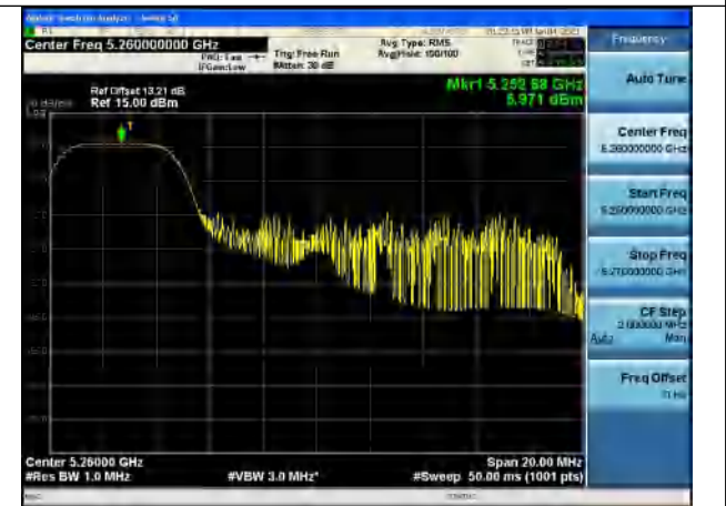
Test Mode:802.11ax HE20 5260MHz Chain1
