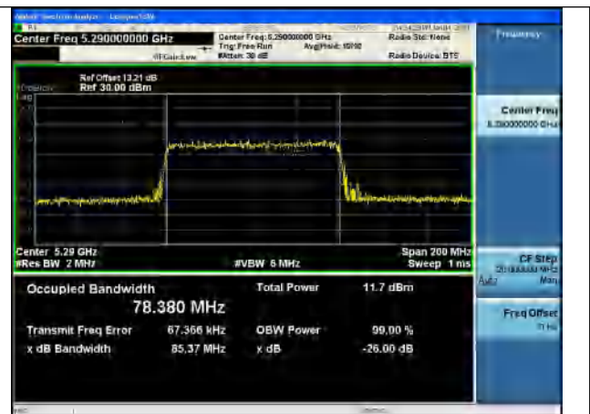
Test Mode:802.11ax HE80 5290MHz Chain1
