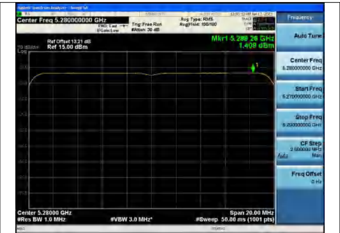
Test Mode:802.11be EHT20 5280MHz Chain0
