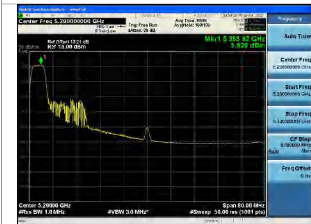
Test Mode:802.11ax HE80 5290MHz Chain0
