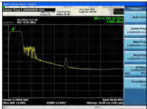
Test Mode:802.11ax HE80 5290MHz Chain1
