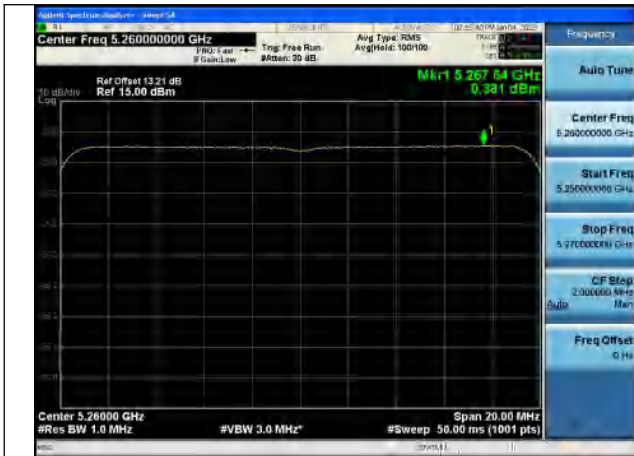
Test Mode:802.11ax HE20 5260MHz Chain0
