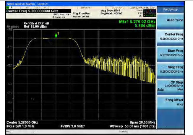
Test Mode:802.11be HE20 5280MHz Chain0
