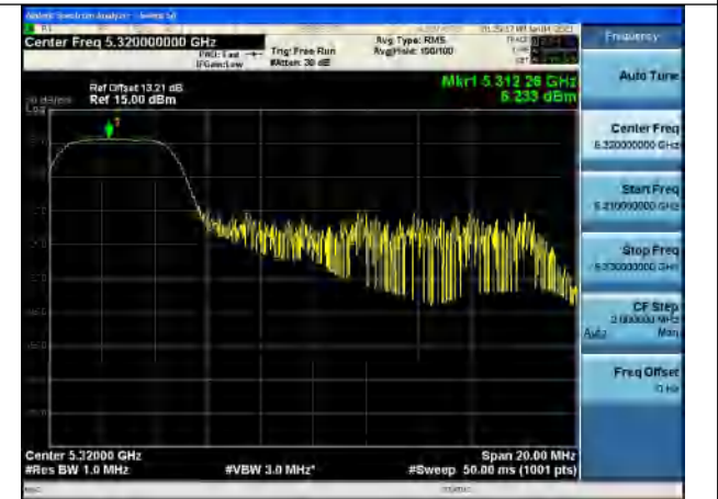
Test Mode:802.11ax HE20 5320MHz Chain1
