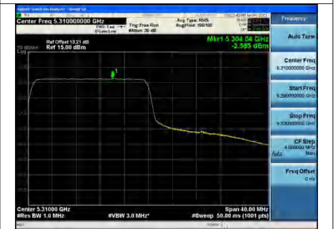
Test Mode:802.11ax HE40 5310MHz Chain1
