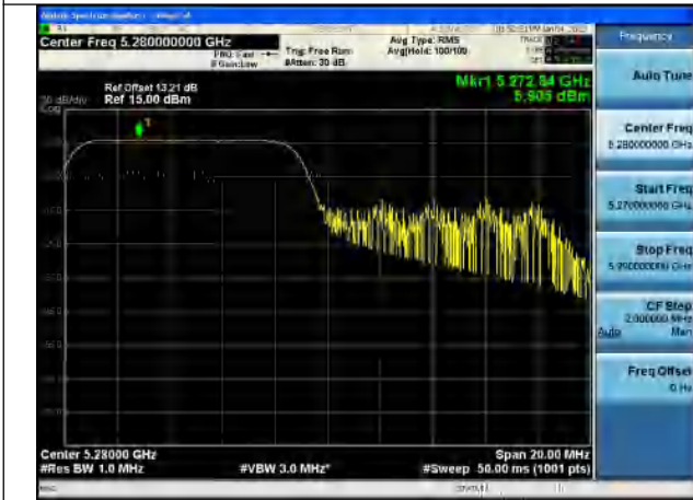
Test Mode:802.11ax HE20 5280MHz Chain1
