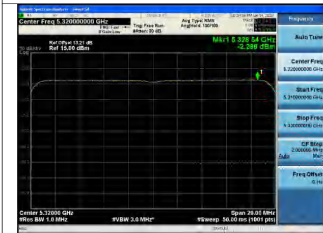
Test Mode:802.11ax HE20 5320MHz Chain0
