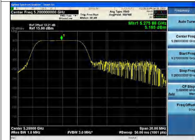
Test Mode:802.11be HE20 5280MHz Chain1
