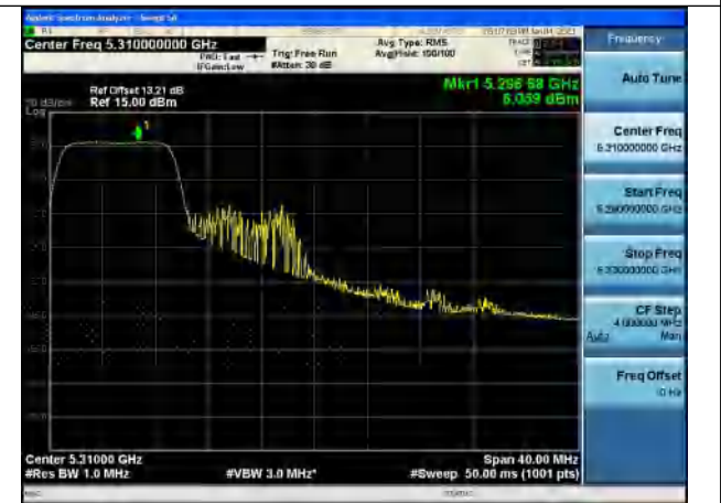
Test Mode:802.11ax HE40 5310MHz Chain0
