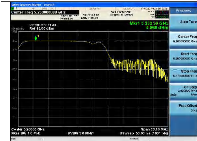
Test Mode:802.11be HE20 5260MHz Chain0
