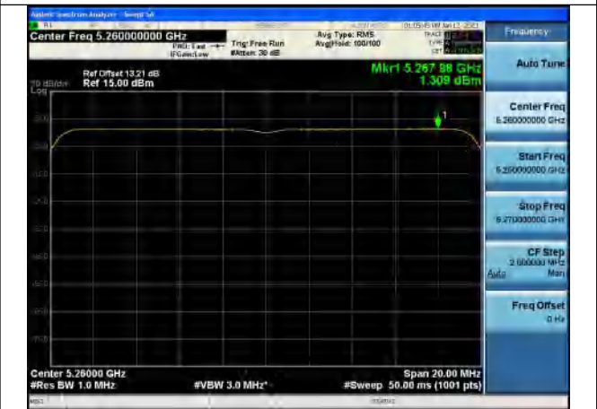
Test Mode:802.11be EHT20 5260MHz Chain1
