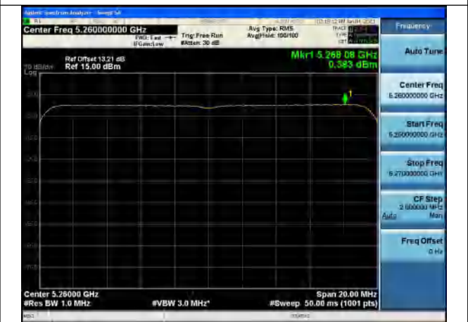
Test Mode:802.11ax HE20 5260MHz Chain1
