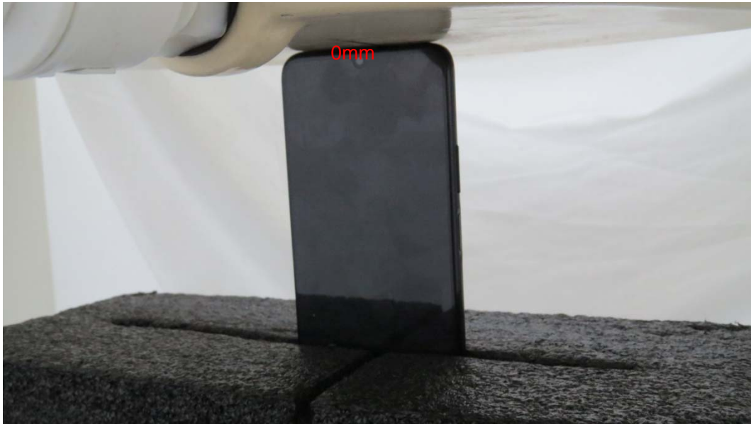
Picture 13: Top Side, the distance from handset to the bottom of the Phantom is 0mm
