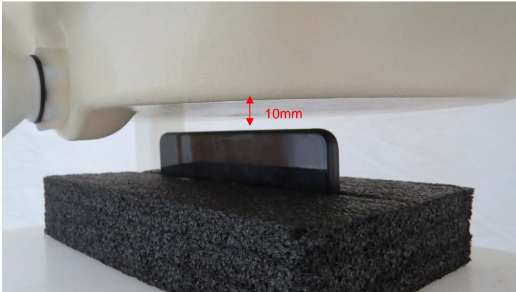
Picture 9: Left Side, the distance from handset to the bottom of the Phantom is 10mm
