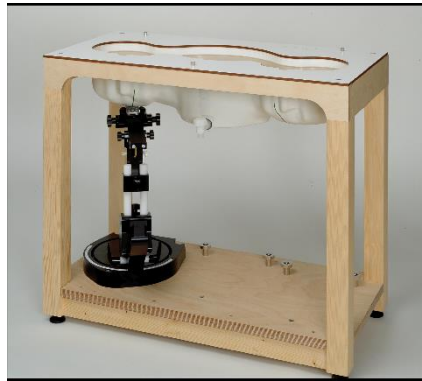
Picture C.8: SAM Twin Phantom
