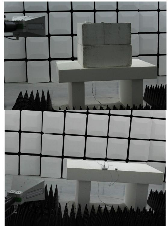
**1.3** Setup for Unwanted Emissions that fall Outside of the Restricted Bands(Radiated) and Unwanted Emissions in the Restricted Bands (Radiated) above 1GHz
