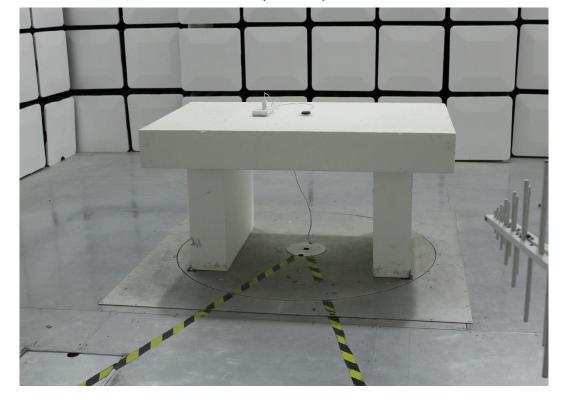
**1.2** Setup for Unwanted Emissions that fall Outside of the Restricted Bands(Radiated) and Unwanted Emissions in the Restricted Bands (Radiated) below 1GHz
