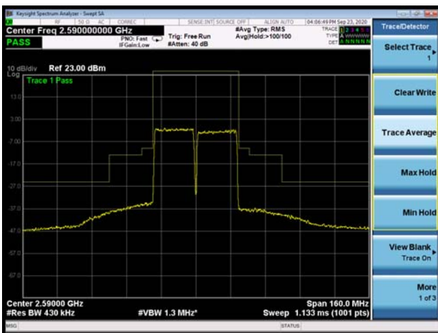
CA_38C 64QAM 20MHz+20MHz CH-Low, 100%RB
