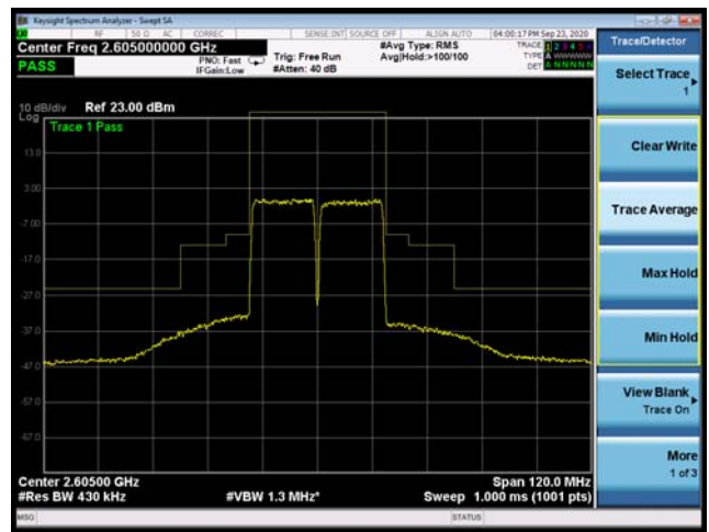
CA_38C 64QAM 15MHz+15MHz CH-High, 1 RB
