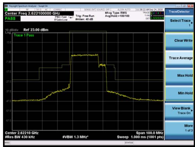
CA_41C 16QAM 20MHz+5MHz CH-High, 1 RB
