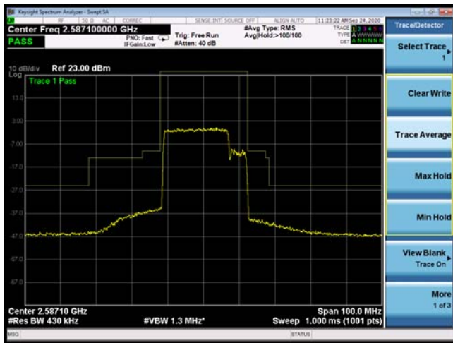
CA_41C 64QAM 20MHz+5MHz CH-Low, 1 RB
