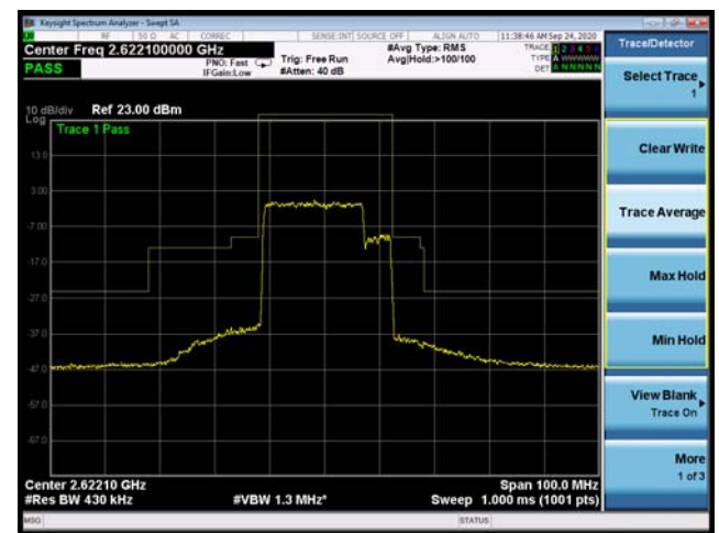
CA_41C 64QAM 20MHz+5MHz CH-High, 100%RB
