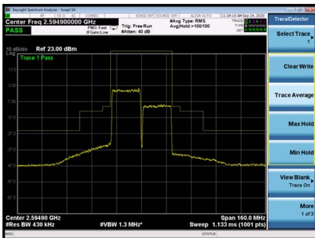
CA_41C 16QAM 20MHz+20MHz CH-Low, 1 RB
