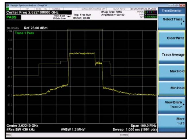
CA_41C 64QAM 20MHz+5MHz CH-High, 1 RB
