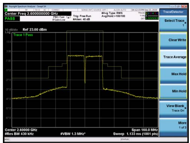
CA_38C 64QAM 20MHz+20MHz CH-High, 100%RB
