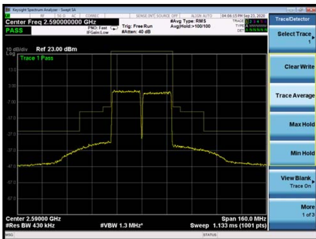
CA_38C 16QAM 20MHz+20MHz CH-Low, 1 RB
