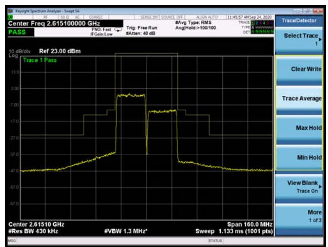
CA_41C 64QAM 20MHz+20MHz CH-High, 100%RB
