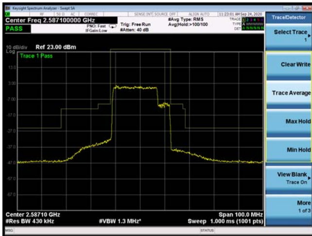
CA_41C 16QAM 20MHz+5MHz CH-Low, 1 RB
