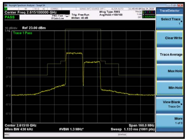
CA_41C 64QAM 20MHz+20MHz CH-High, 1 RB
