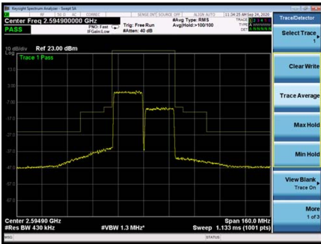
CA_41C 64QAM 20MHz+20MHz CH-Low, 1 RB
