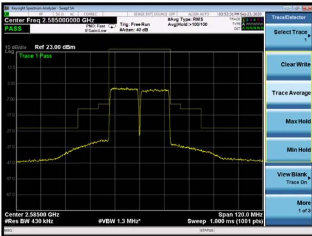
CA_38C 64QAM 15MHz+15MHz CH-Low, 1 RB
