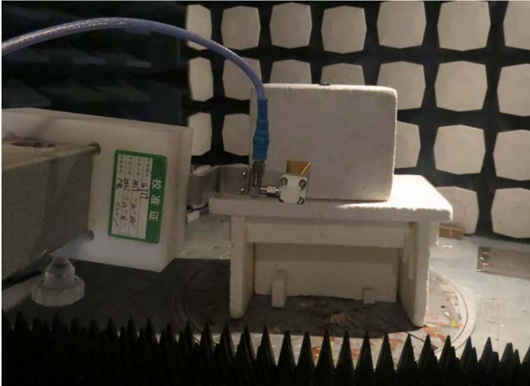
Picture 1: Radiated Spurious Emissions Test setup
