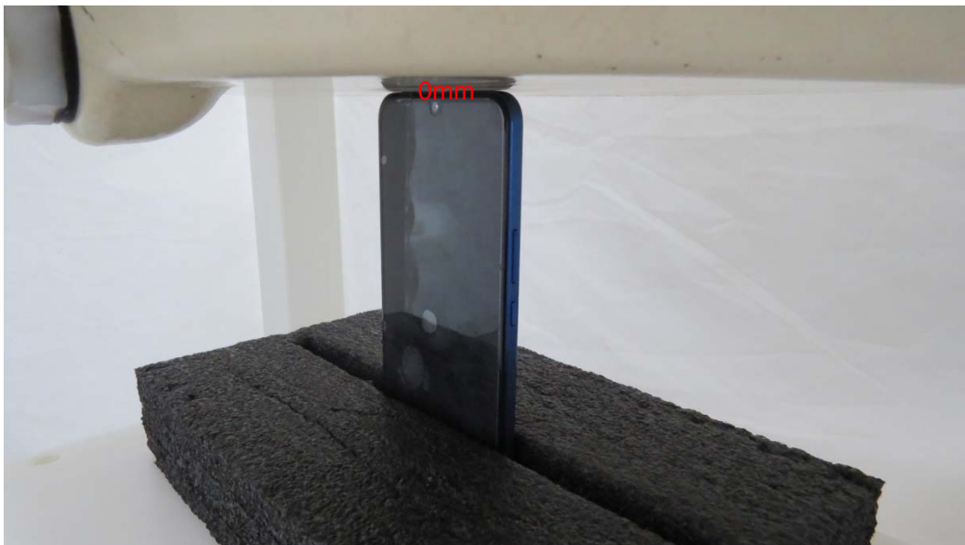
Picture 16: Top Side, the distance from handset to the bottom of the Phantom is 0mm
