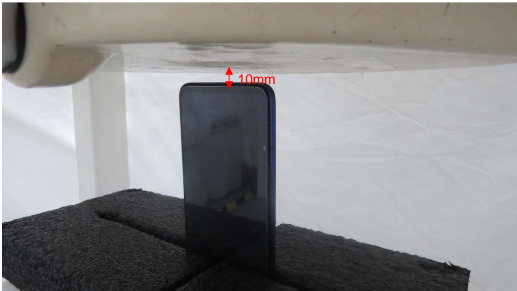
Picture 12: Bottom Edge, the distance from handset to the bottom of the Phantom is 10mm
