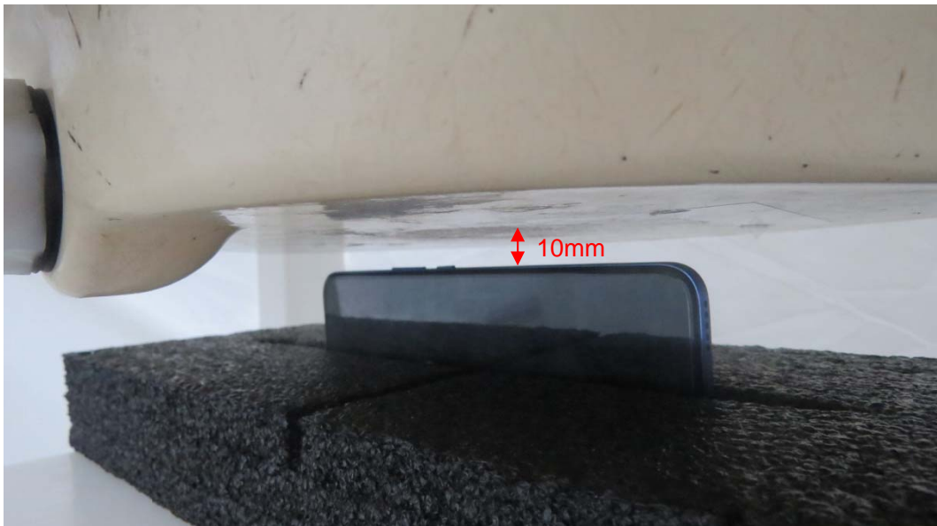
Picture 10: Right Side, the distance from handset to the bottom of the Phantom is 10mm
