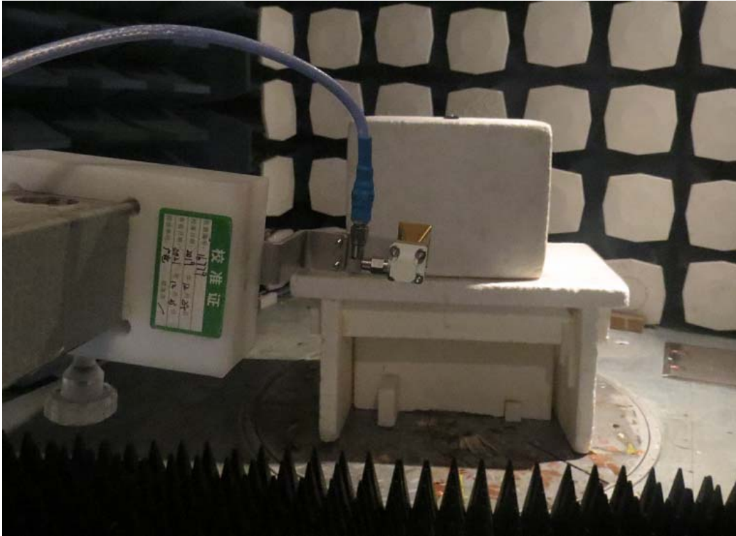
Picture 1: Radiated Spurious Emissions Test setup
