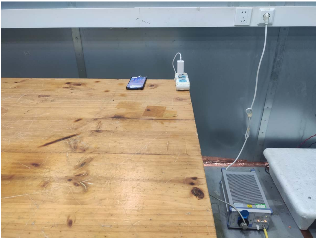
Picture 2 Conducted Emission Test Setup
