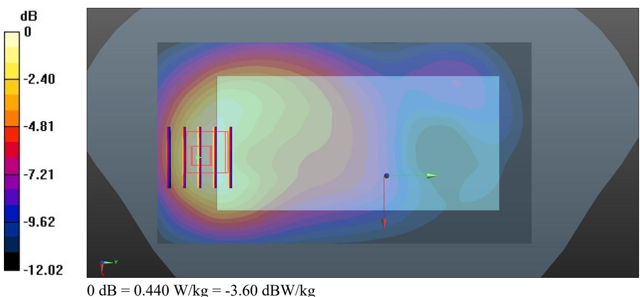
**55\_LTE Band 25\_20M\_QPSK\_50RB\_0Offset\_Back\_15mm\_Ch26340**
