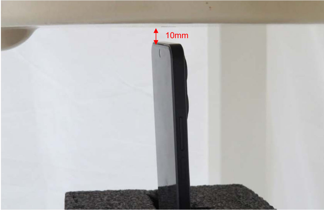
Picture 11: Top Edge, the distance from handset to the bottom of the Phantom is 10mm
