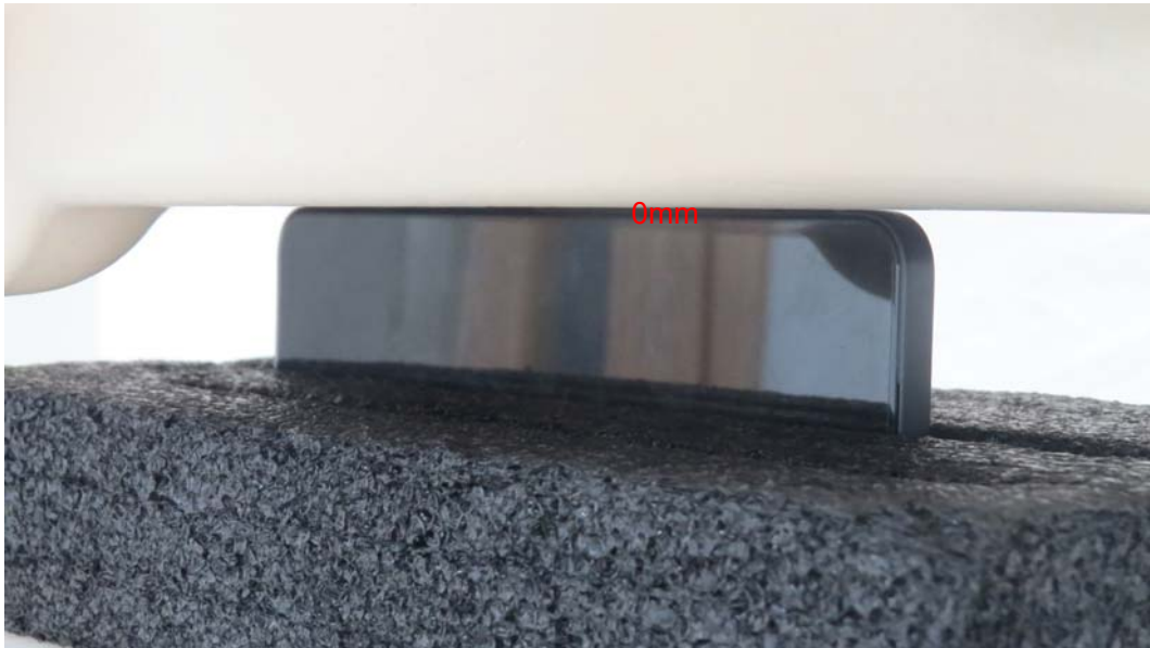
Picture 15: Left Edge, the distance from handset to the bottom of the Phantom is 0mm
