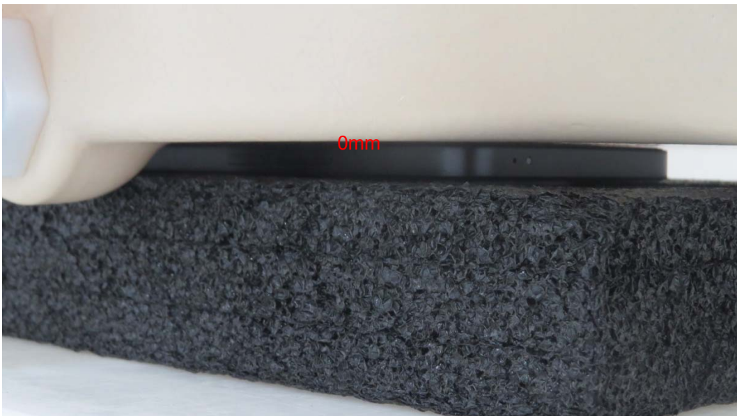
Picture 14: Front Side, the distance from handset to the bottom of the Phantom is 0mm
