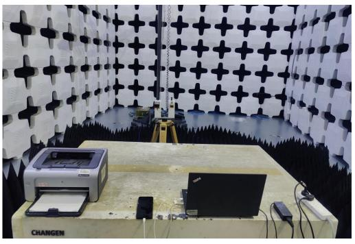
4. Radiated Emissions (Part 15B, Data Transfer, 26.5GHz-40GHz)
