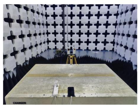
7. Radiated Emissions (Part 15B, Camera/Video Player/GSM receiver/WCDMA receiver/LTE receiver,18GHz-26.5GHz)
