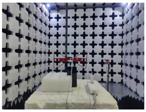
15. Radiated Emissions (Part 15C&Part 15E, 1GHz -18GHz)
