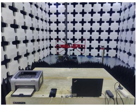
2. Radiated Emissions (Part 15B, Data Transfer, 1GHz-18GHz)
