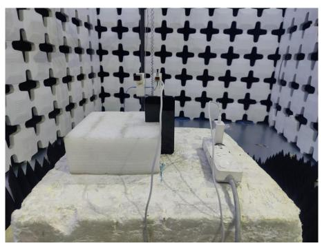
17. Radiated Emissions (Part 15C&Part 15E, 26.5GHz -40GHz)
