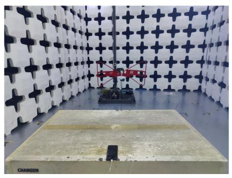
9. Radiated Emissions (Part 15B, FM receiver, 30MHz-1GHz)
