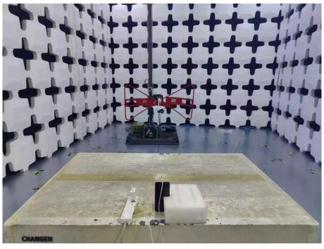
14. Radiated Emissions (Part 15C&Part 15E,30MHz-1GHz)
