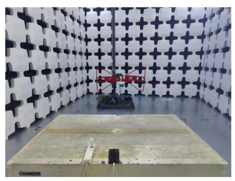
5. Radiated Emissions (Part 15B, Camera/Video Player/GSM receiver/WCDMA receiver/LTE receiver,30MHz-1GHz)
