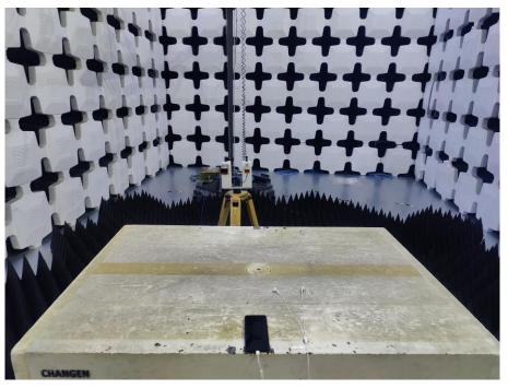
12. Radiated Emissions (Part 15B, FM receiver, 26.5GHz-40GHz)
