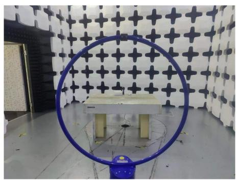
13. Radiated Emissions (Part 15C&Part 15E, 9kHz-30MHz)
