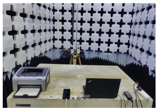
3. Radiated Emissions (Part 15B, Data Transfer, 18GHz-26.5GHz)
