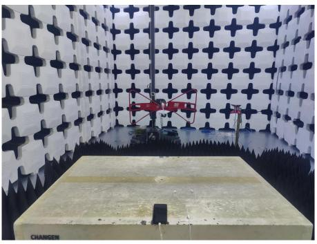
10. Radiated Emissions (Part 15B, Camera/Video Player/GSM receiver/WCDMA receiver/LTE receiver,1GHz-18GHz)
