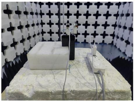
16. Radiated Emissions (Part 15C&Part 15E, 18GHz -26.5GHz)
