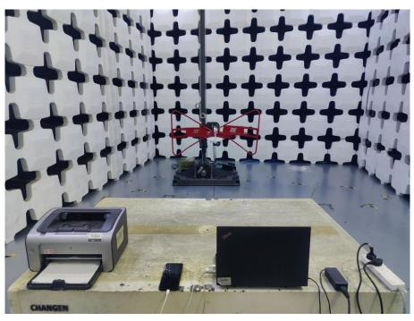
1. Radiated Emissions (Part 15B, Data Transfer, 30MHz-1GHz)
