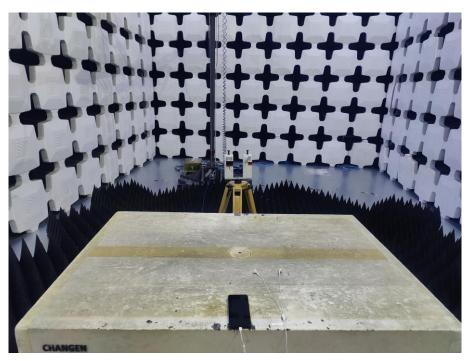
11. Radiated Emissions (Part 15B, FM receiver, 18GHz-26.5GHz)
