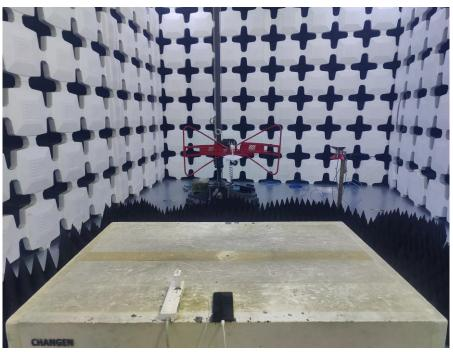
6. Radiated Emissions (Part 15B, Camera/Video Player/GSM receiver/WCDMA receiver/LTE receiver,1GHz-18GHz)
