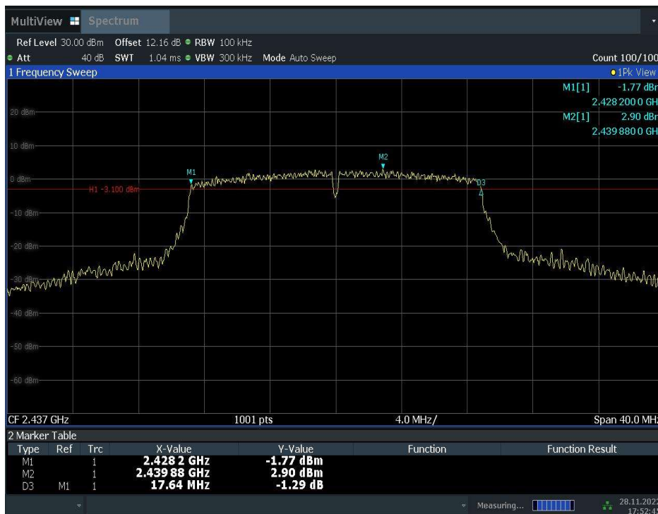
Fig.A.4.8 Occupied 6dB Bandwidth (802.11n-HT20, Ch 6)
