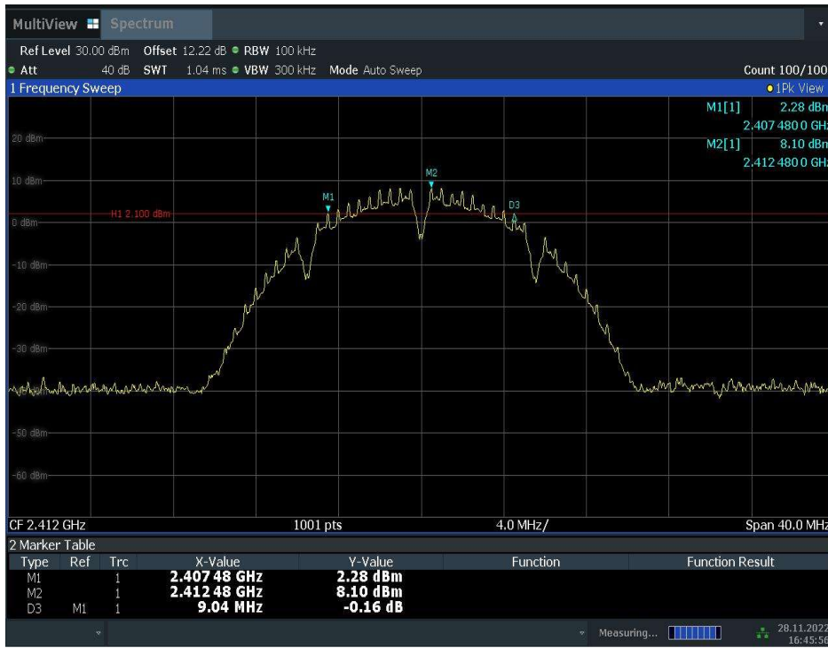
Fig.A.4.1 Occupied 6dB Bandwidth(802.11b,Ch 1)
