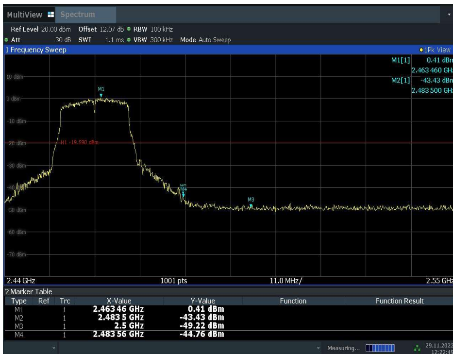
Fig.A.5.4 Band Edges (802.11g, Ch 11)
