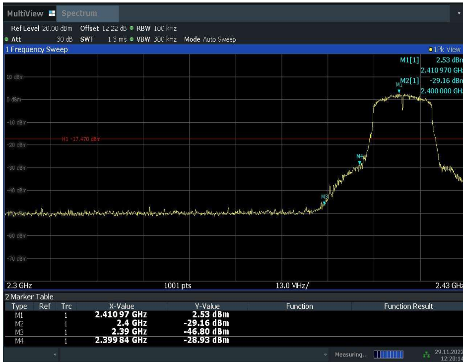
Fig.A.5.3 Band Edges (802.11g, Ch 1)
