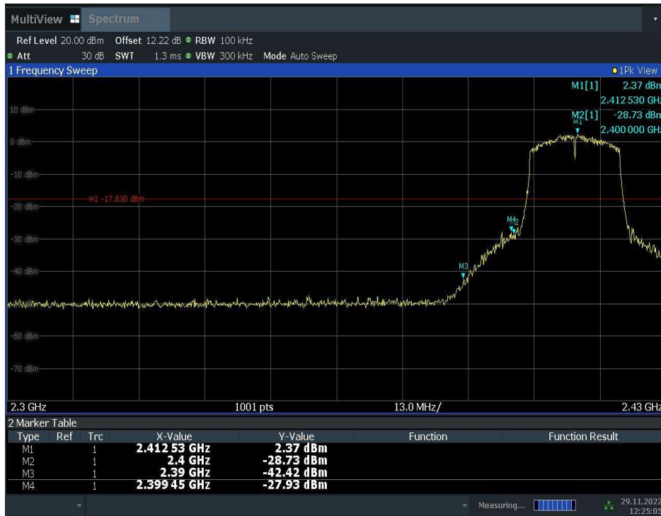
Fig.A.5.5 Band Edges (802.11n-HT20, Ch 1)
