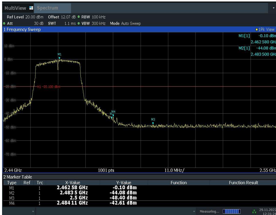
Fig.A.5.6 Band Edges (802.11n-HT20, Ch 11)
