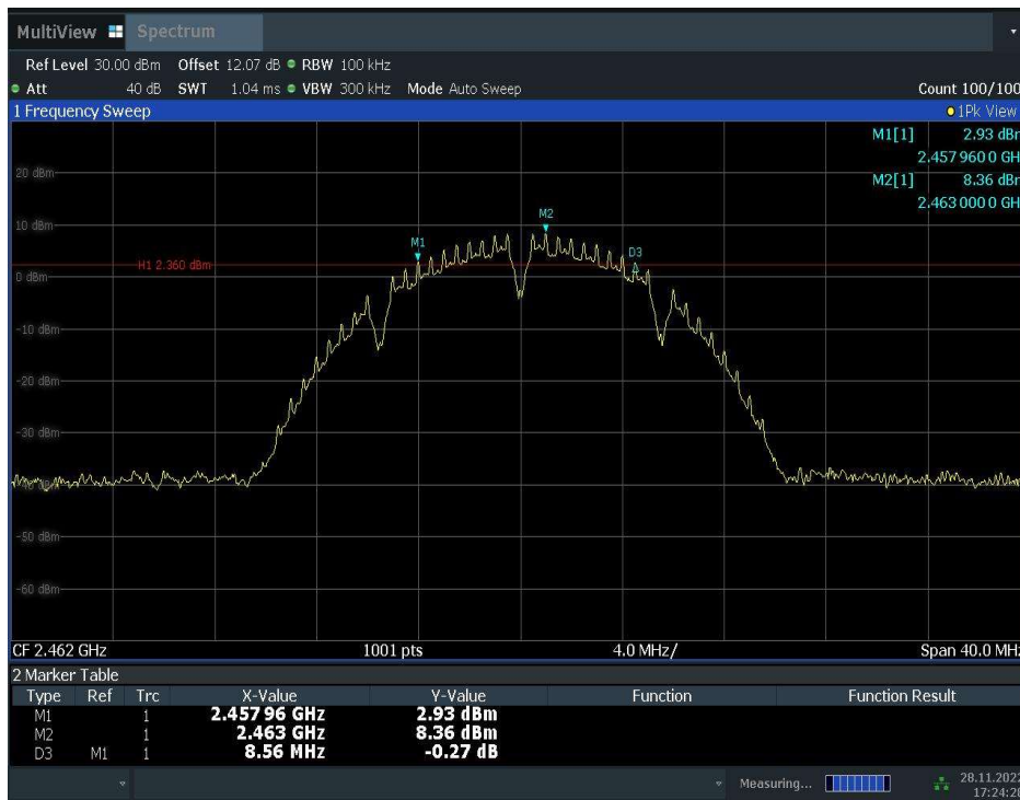
Fig.A.4.3 Occupied 6dB Bandwidth (802.11b, Ch 11)
