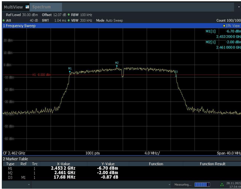
Fig.A.4.9 Occupied 6dB Bandwidth (802.11n-HT20, Ch 11)
