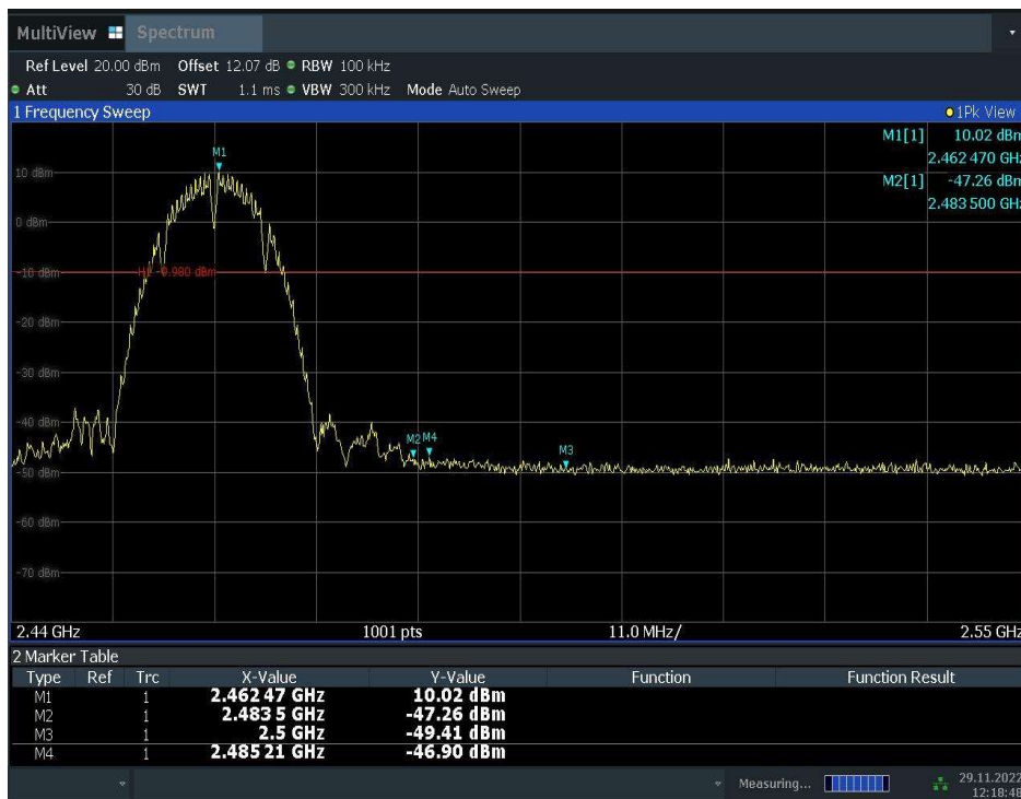
Fig.A.5.2 Band Edges (802.11b, Ch 11)
