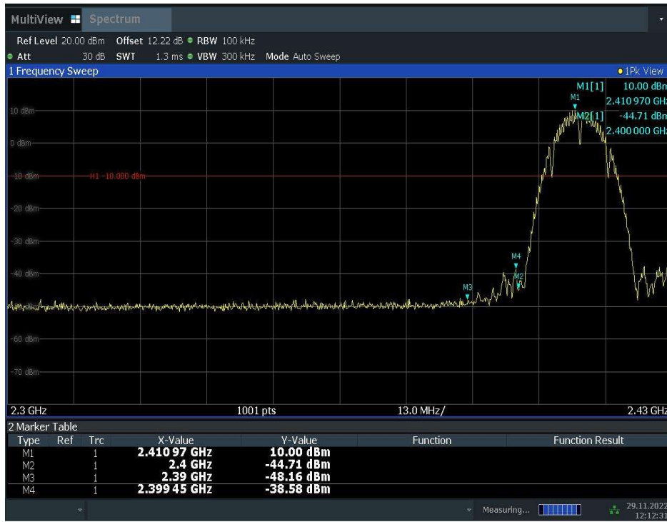
Fig.A.5.1 Band Edges (802.11b, Ch 1)
