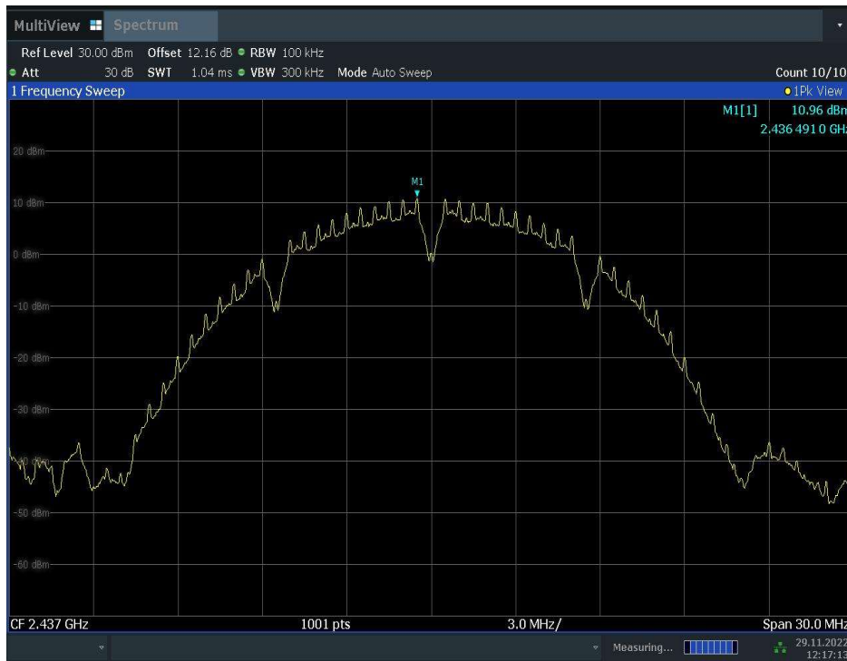
Fig.A.6.1.4 Transmitter Spurious Emission - Conducted (802.11b, Ch6, Center Frequency)
