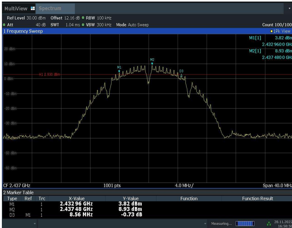
Fig.A.4.2 Occupied 6dB Bandwidth (802.11b, Ch 6)
