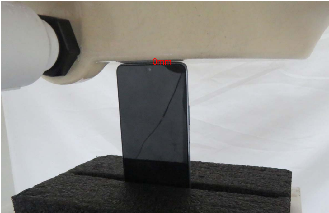
Picture 17: Top Edge, the distance from handset to the bottom of the Phantom is 0mm
