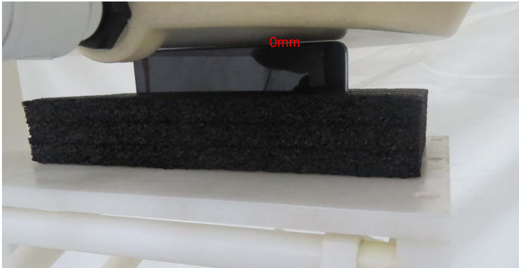
Picture 15: Left Edge, the distance from handset to the bottom of the Phantom is 0mm
