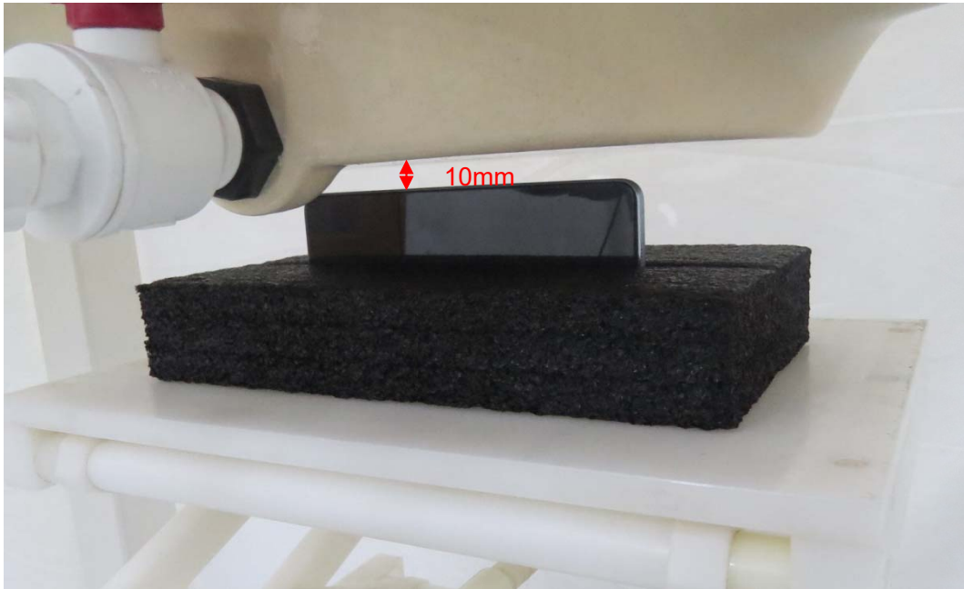
Picture 9: Left Edge, the distance from handset to the bottom of the Phantom is 10mm
