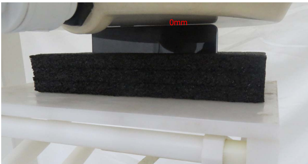
Picture 16: Right Edge, the distance from handset to the bottom of the Phantom is 0mm
