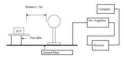
Semi-Anechoic 3m Chamber
