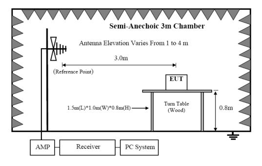
In 3m Anechoic Chamber Test Setup Diagram for frequency 30MHz-1GHz
