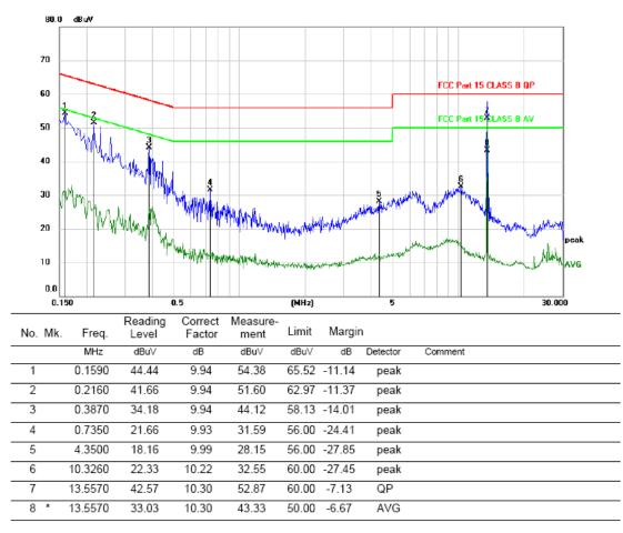
Note: Measurement=Reading Level+Correc Factor. Factor=(LISN or ISN or PLC or Current Probe)Factor+Cable
