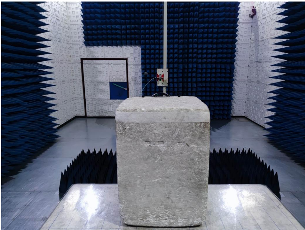
RADIATED EMISSION TEST SETUP ABOVE 1GHz
