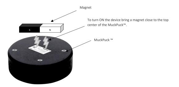
2. Once the MuckPuck<sup>™</sup> device is ON, it would automatically broadcast its location and other sensor data periodically and when motion detected. The MuckPuck<sup>™</sup> device data can be received and comprehend by Peytec's compatible readers.
