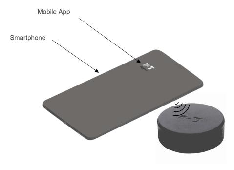
4. To update the MuckPuck<sup>™</sup> status, simply make the changes as you wish on Peytec's mobile app and click on "Upload" and wait for the confirmation message on your mobile phone confirming the MuckPuck<sup>™</sup> Device is programmed.
