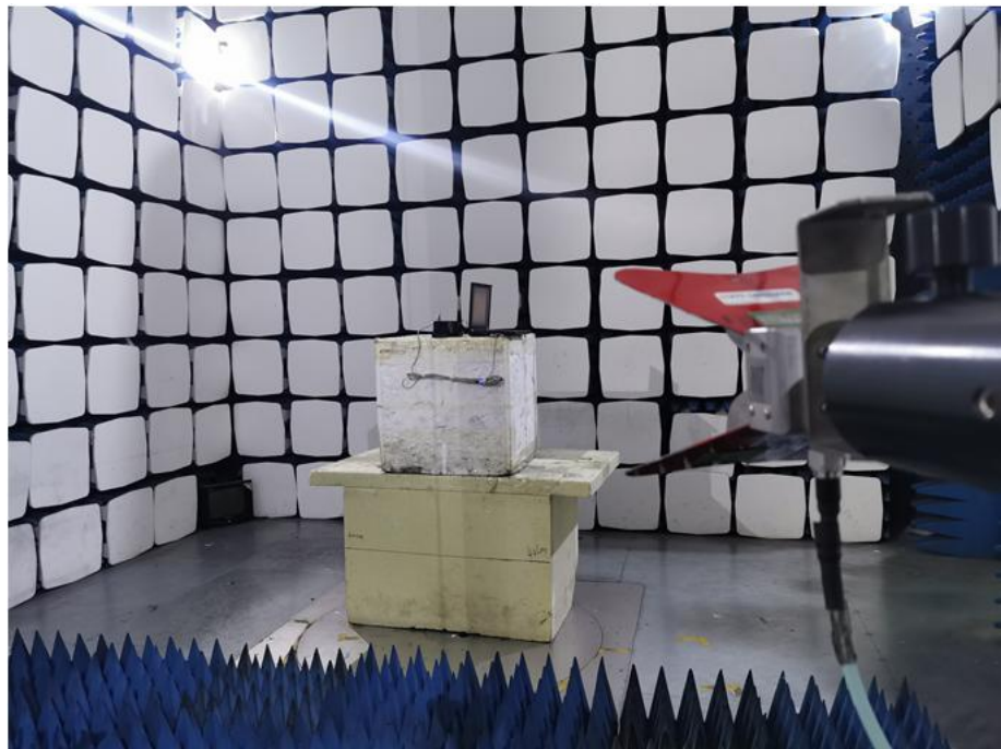
Radiation Emission Test Setup (1GHz to 18GHz)
