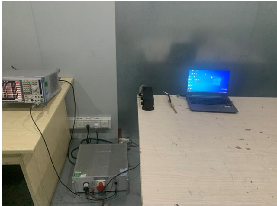
Conducted Emission Test Setup
