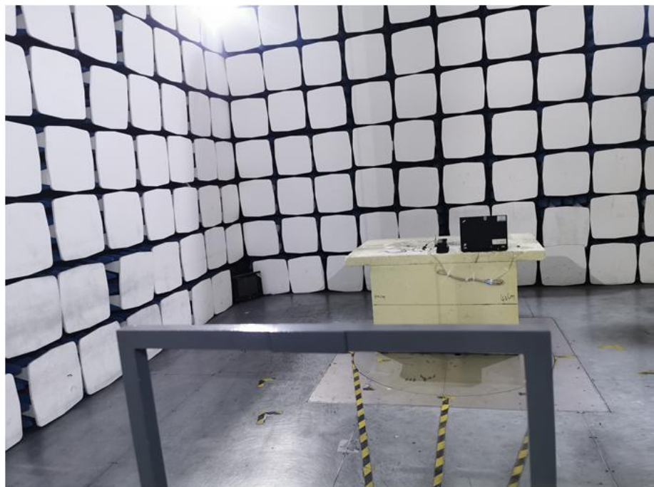
Radiation Emission Test Setup (Below 30MHz)
