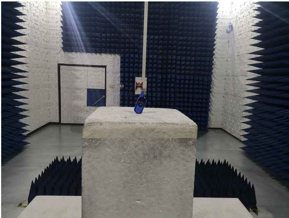
RADIATED EMISSION ABOVE 1G TEST SETUP
