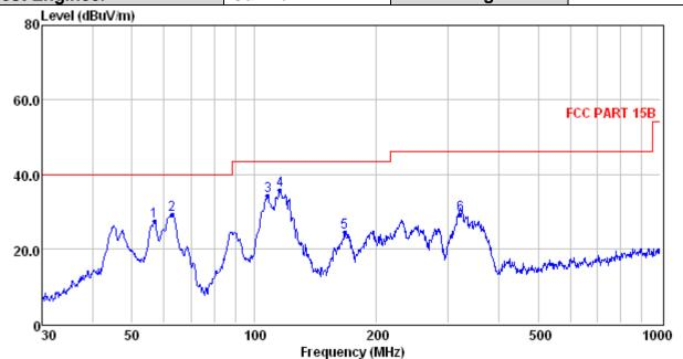
Reading CabLos Antfac Measured Limit Over Remark MHzdBuV dΒ dB/m dBuV/m dBuV/m dB 1 56.79 43.93 0.47 12.90 27.27 40.00 -12.73QP 2 62.87 47.14 0.48 11.55 29.12 40.00 -10.88 QP 3 107.89 51.23 0.68 12.44 34.22 -9.28 43.50 QP -7.96 4 115.73 53.77 0.68 11.24 35.54 43.50 QP 5 167.24 44.96 0.77 8.89 24.33 43.50 -19.17QP 322.19 45.00 1.16 13.42 29.00 46.00 -17.00 QP
