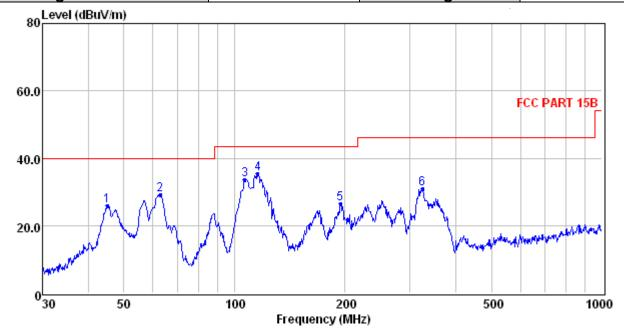
Limit Freq Reading CabLos Antfac Measured Over Remark MHzdBuV dΒ dB/m dBuV/m dBuV/m dΒ 41.96 45.06 0.41 13.55 25.93 40.00 -14.07 1 2 47.18 62.87 0.48 11.55 29.16 40.00 -10.84QP 3 106.76 50.58 0.68 12.54 33.68 43.50 -9.82 QP 4 115.73 53.54 0.68 11.24 35.31 43.50 -8.19 QΡ 5 194.45 45.54 0.76 10.56 26.52 43.50 -16.98 QP 324.46 46.82 1.10 13.51 30.84 46.00 -15.16QP
